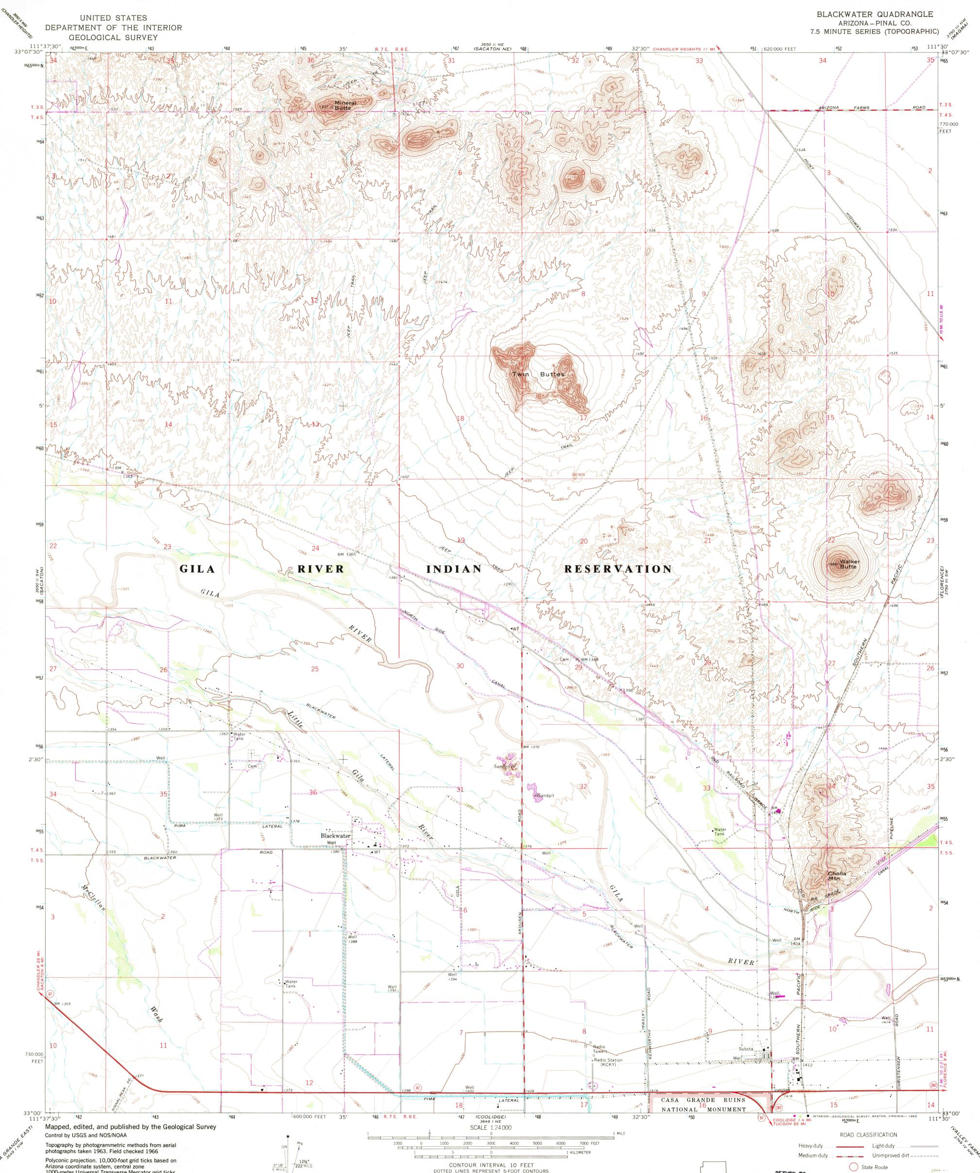
Polyconic projection. 10,000-foot grid ticks based on Arizona coordinate system, central zone 1000-meter Universal Transverse Mercator grid ticks, zone 12, shown in blue. 1927 North American Datum To place on the predicted North American Datum 1983 move the projection lines 2 meters south and move the projection lines 2 meters south and 63 meters east as shown by dashed corner ticks
