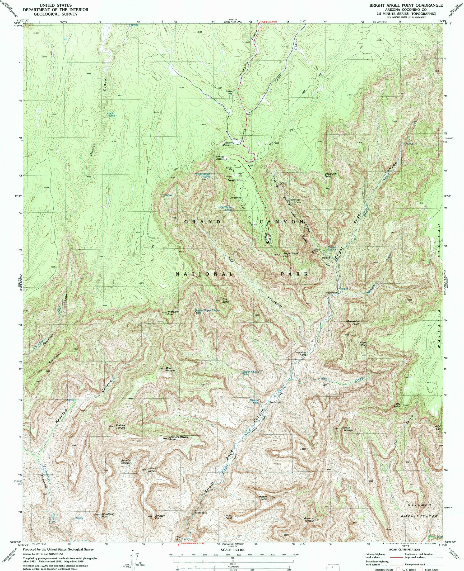
1000-meter Universal Transverse Mercator grid, zone 12 1927 North American Datum To place on the predicted North American Datum 1983 move the projection lines 6 meters north and 66 meters east as shown by dashed corner ticks
