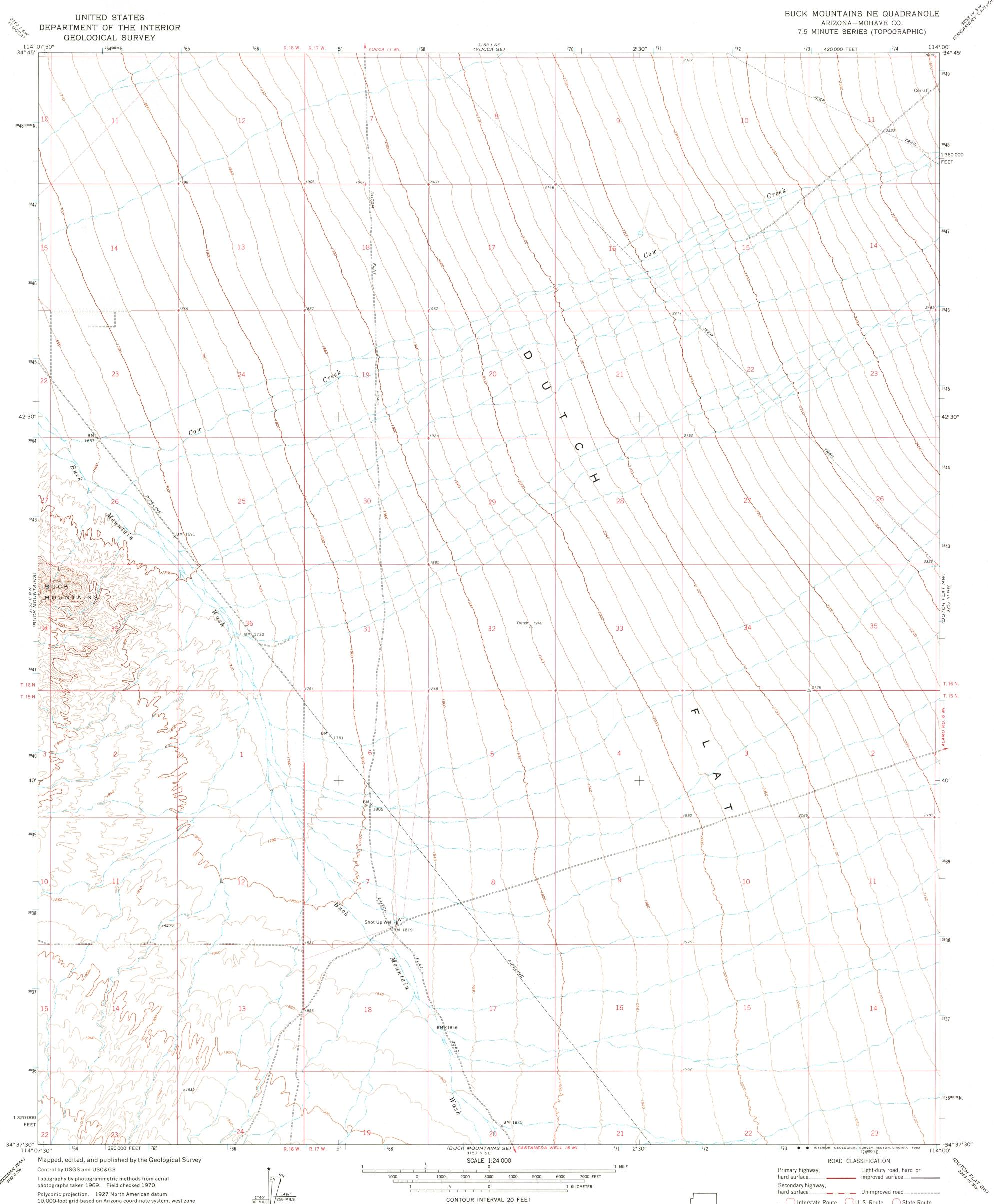
10,000-foot grid based on Arizona coordinate system, west zone 1000-meter Universal Transverse Mercator grid ticks, zone 11, shown in blue To place on the predicted North American Datum 1983 move the projection lines 1 meter north and 72 meters east as shown by dashed corner ticks
