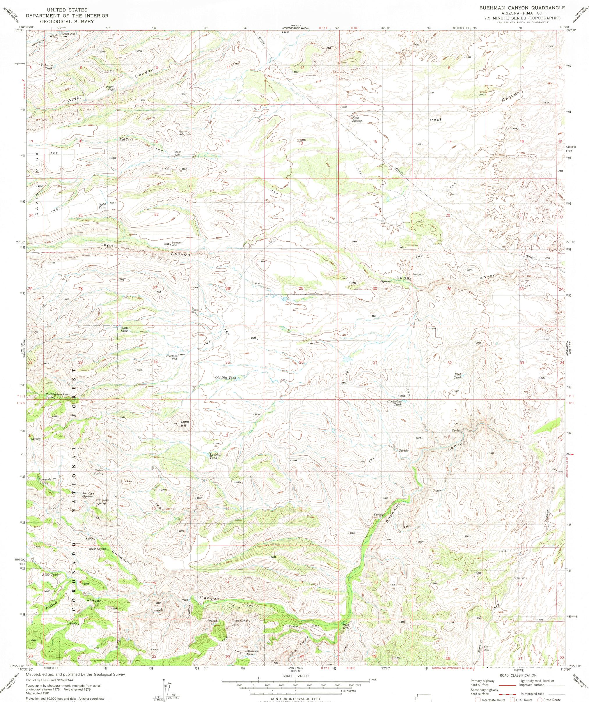
Projection and 10,000-foot grid ticks: Arizona coordinate system, central zone (transverse Mercator) 1000-meter Universal Transverse Mercator grid, zone 12 1927 North American Datum To place on the predicted North American Datum 1983 move the projection lines 6 meters south and 61 meters east as shown by dashed corner ticks There may be private inholdings within the boundaries of the National or State reservations shown on this map
