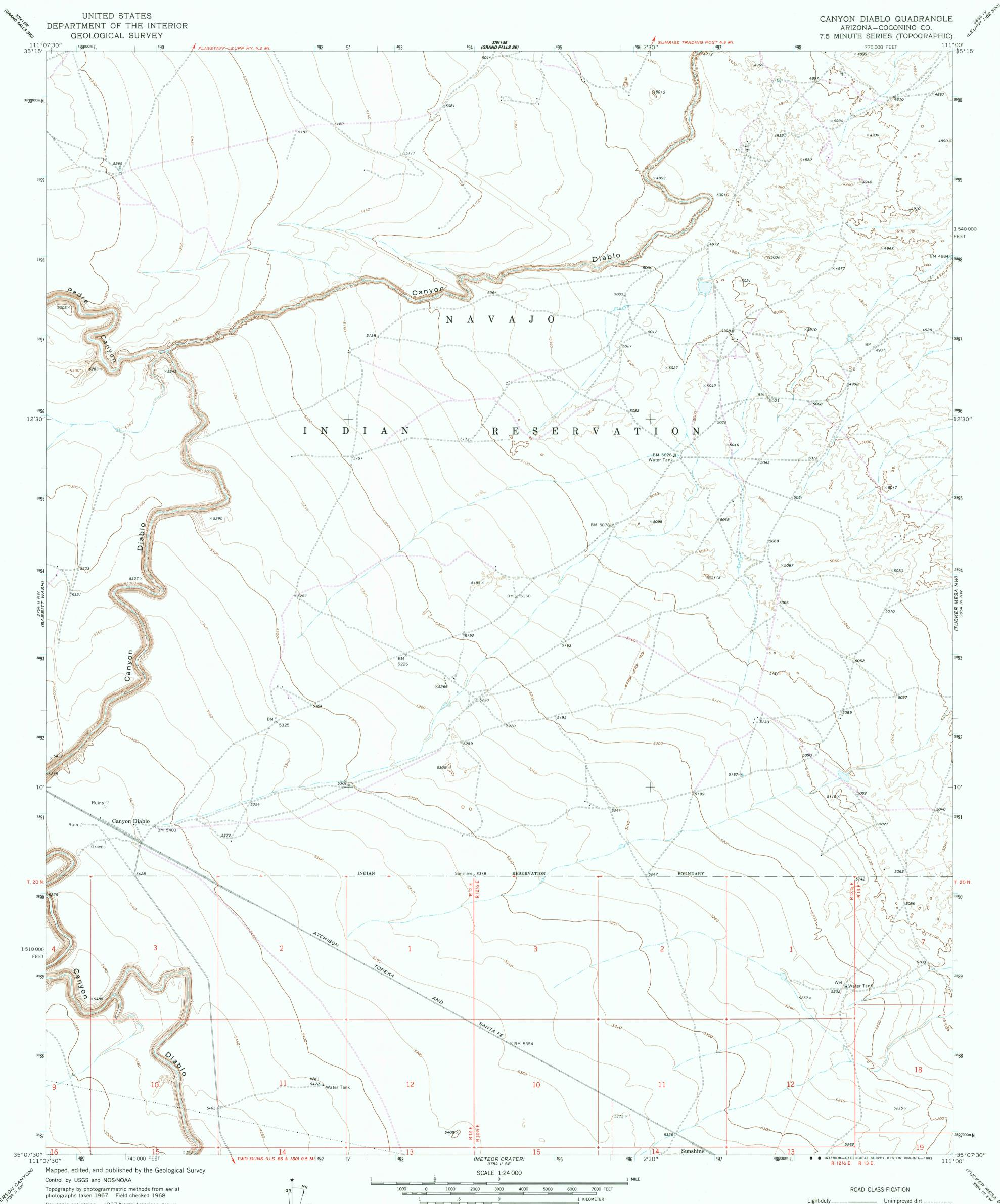
Polyconic projection. 1927 North American datum 10,000-foot grid based on Arizona coordinate system, central zone 1000-meter Universal Transverse Mercator grid ticks, zone 12, shown in blue To place on the predicted North American Datum 1983 move the projection lines 1 meter north and 63 meters east as shown by dashed corner ticks Fine red dashed lines indicate selected fence lines
