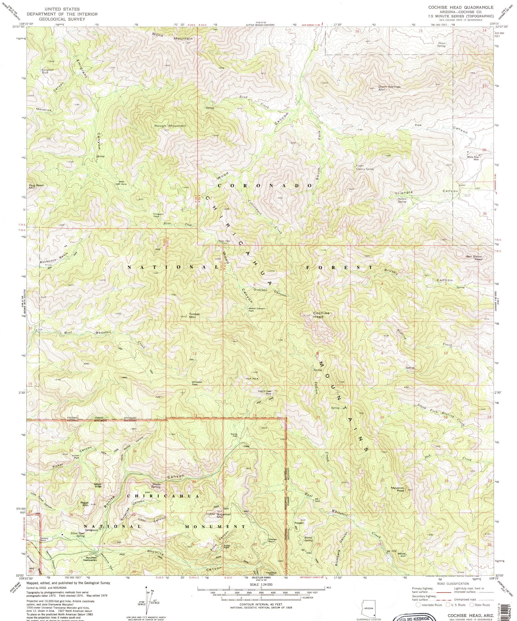
system, east zone (transverse Mercator) 1000-meter Universal Transverse Mercator grid ticks, zone 12, shown in blue. 1927 North American datum To place on the predicted North American Datum 1983 move the projection lines 8 meters south and 58 meters east as shown by dashed corner ticks
