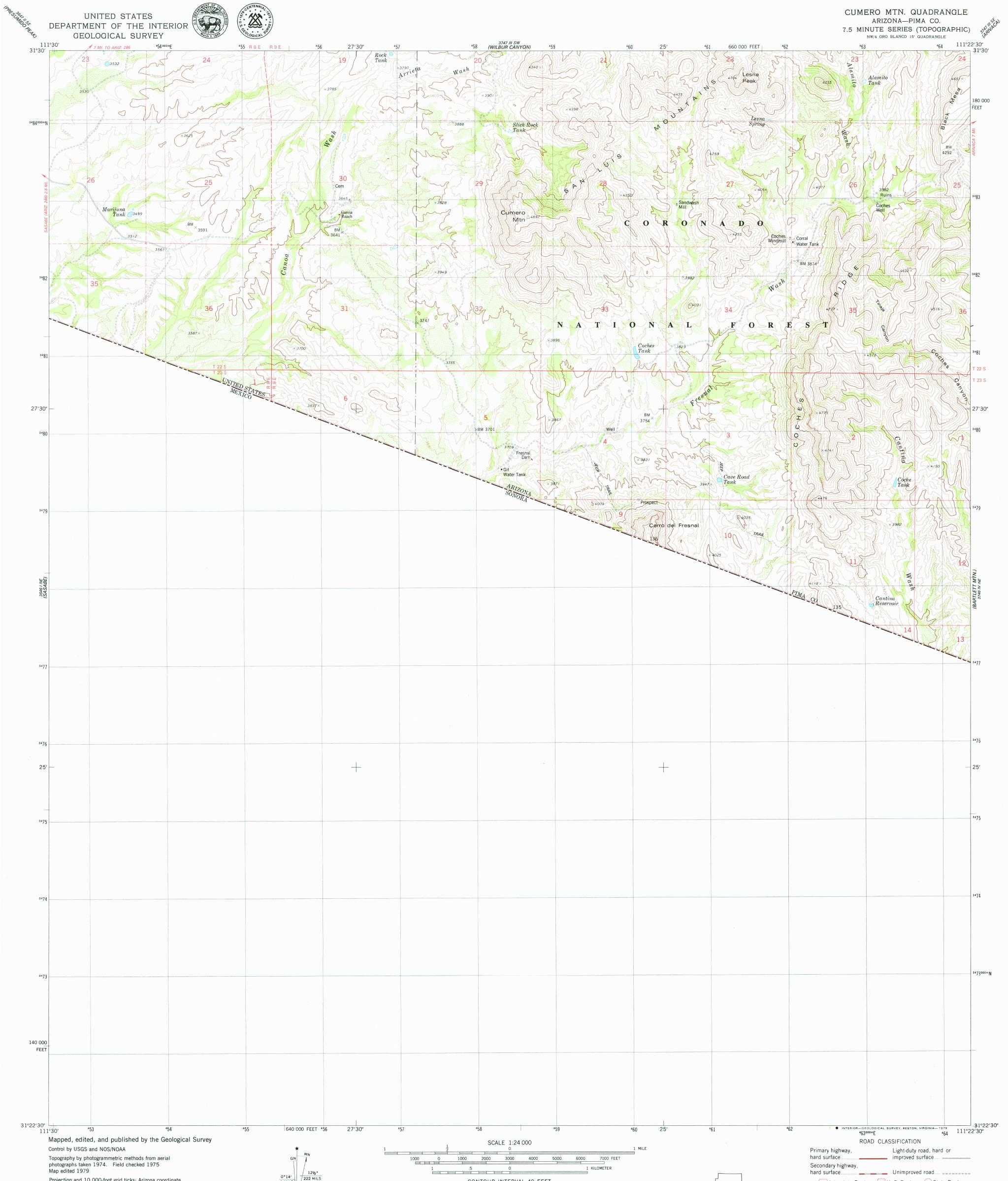
Projection and 10,000-foot grid ticks: Arizona coordinate system, central zone (transverse Mercator) 1000-meter Universal Transverse Mercator grid, zone 12 1927 North American Datum To place on the predicted North American Datum 1983 move the projection lines 9 meters south and 63 meters east as shown by dashed corner ticks There may be private inholdings within the boundaries of the National or State reservations shown on this map
