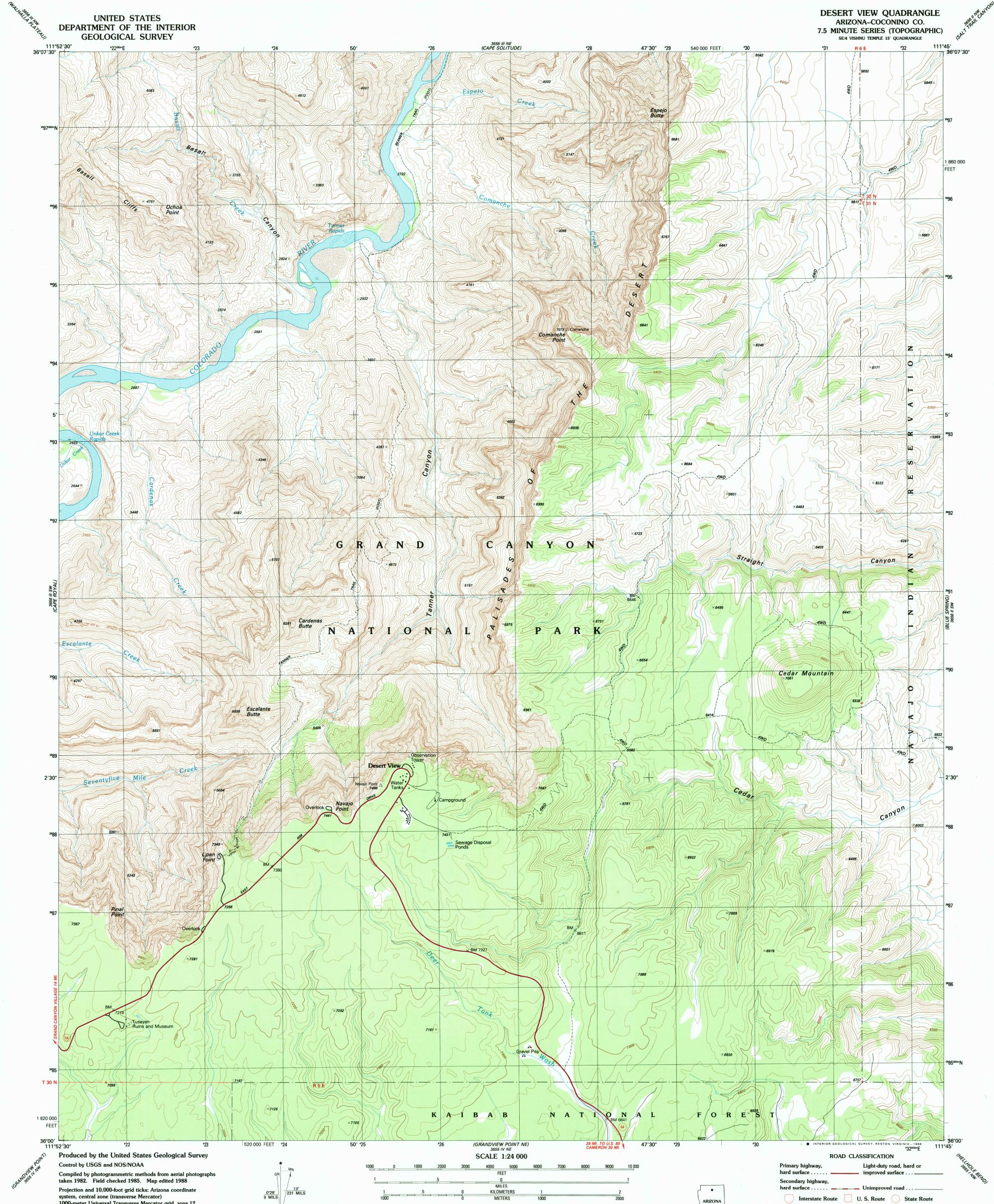
1000-meter Universal Transverse Mercator grid, zone 12 1927 North American Datum To place on the predicted North American Datum 1983 move the projection lines 5 meters north and 65 meters east as shown by dashed corner ticks
