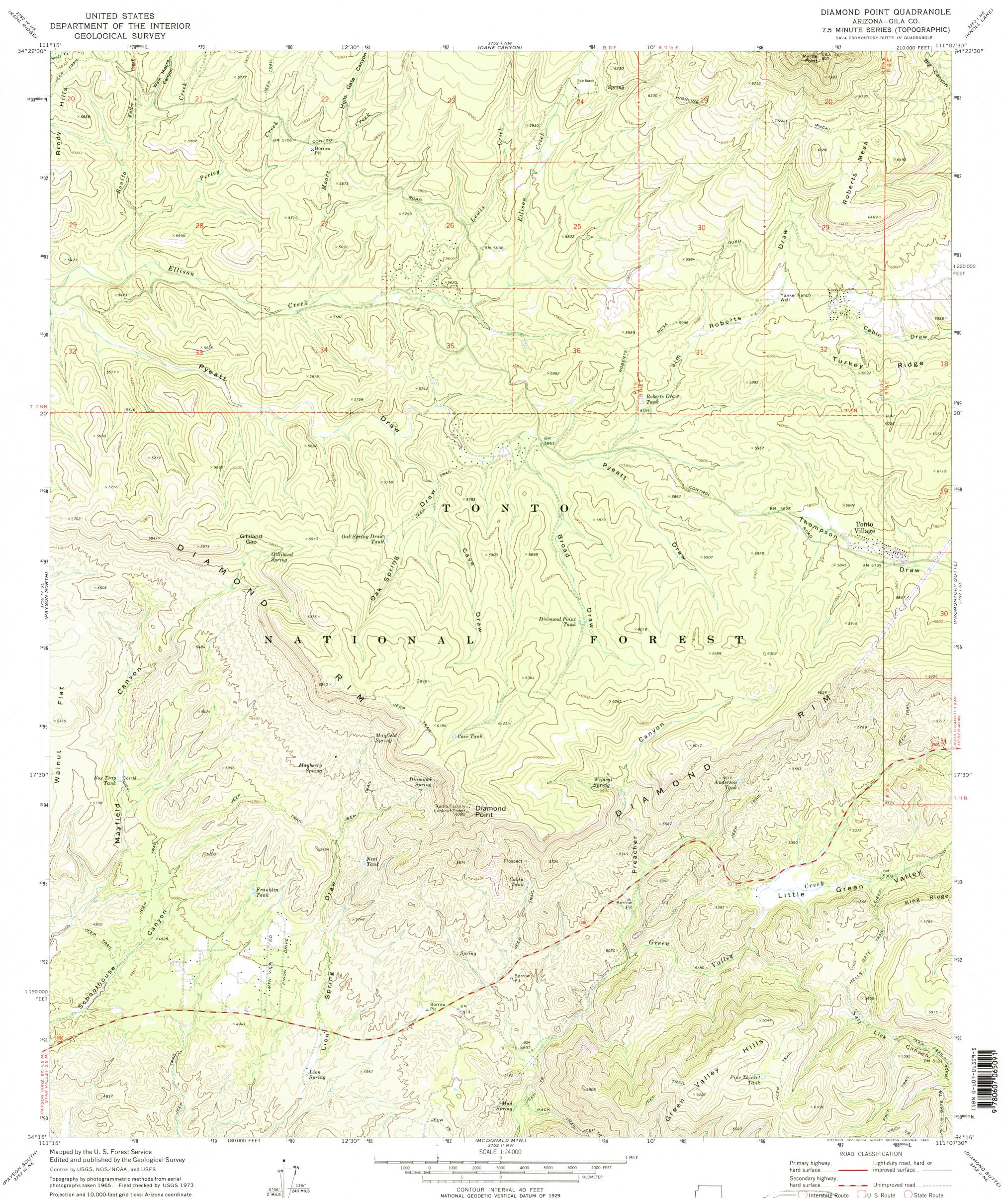
Projection and 10,000-foot grid ticks: Arizona coordinate system, east zone (transverse Mercator) 1000-meter Universal Transverse Mercator grid ticks, zone 12, shown in blue. 1927 North American datum To place on the predicted North American Datum 1983 move the projection lines 1 meter south and 63 meters east as shown by dashed corner ticks Where omitted, land lines have not been established
