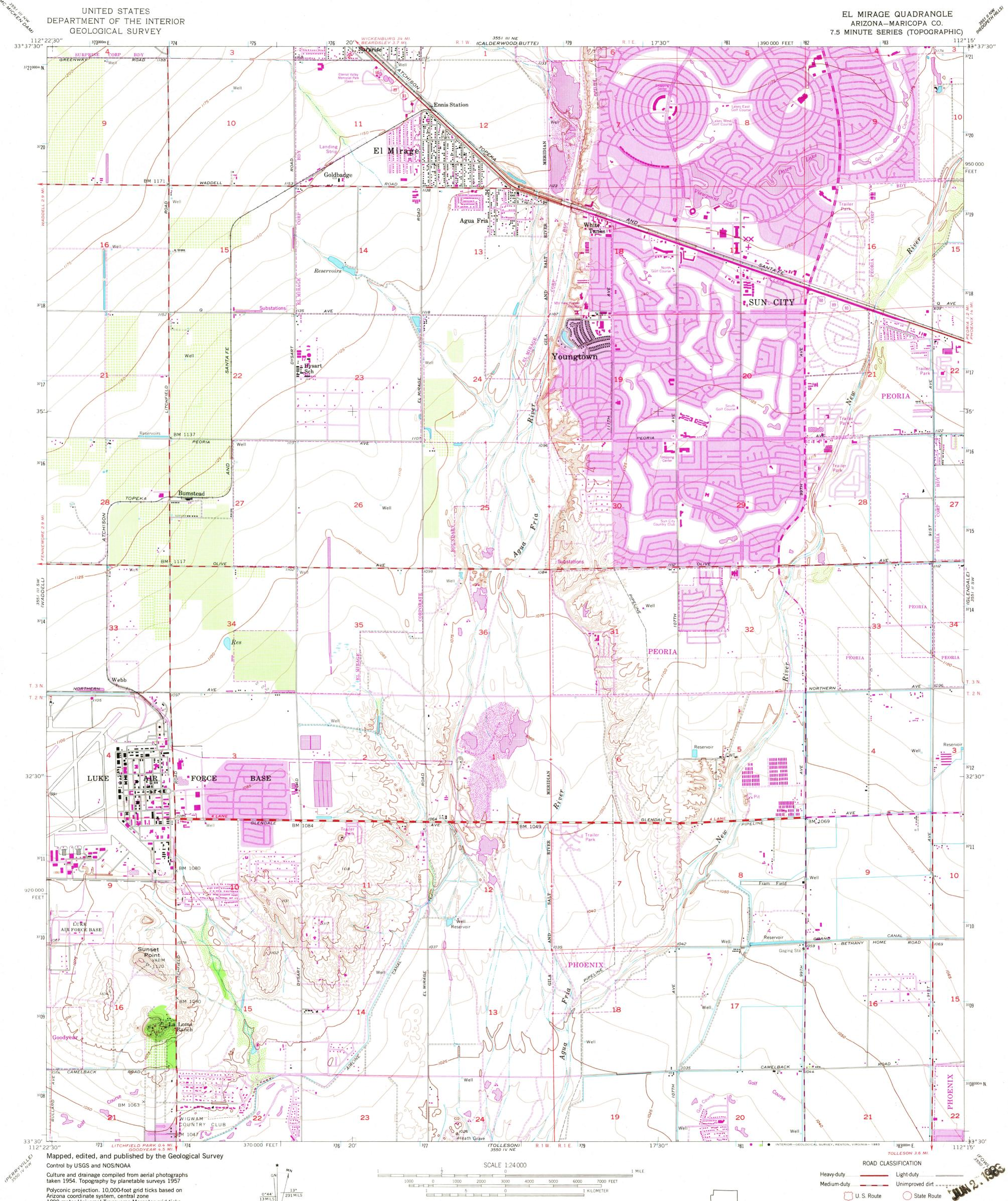
Polyconic projection. 10,000-foot grid ticks based on Arizona coordinate system, central zone 1000-meter Universal Transverse Mercator grid ticks, zone 12, shown in blue. 1927 North American Datum To place on the predicted North American Datum 1983 move the projection lines 2 meters south and 66 meters east as shown by dashed corner ticks There may be private inholdings within the boundaries of the National or State reservations shown on this map
