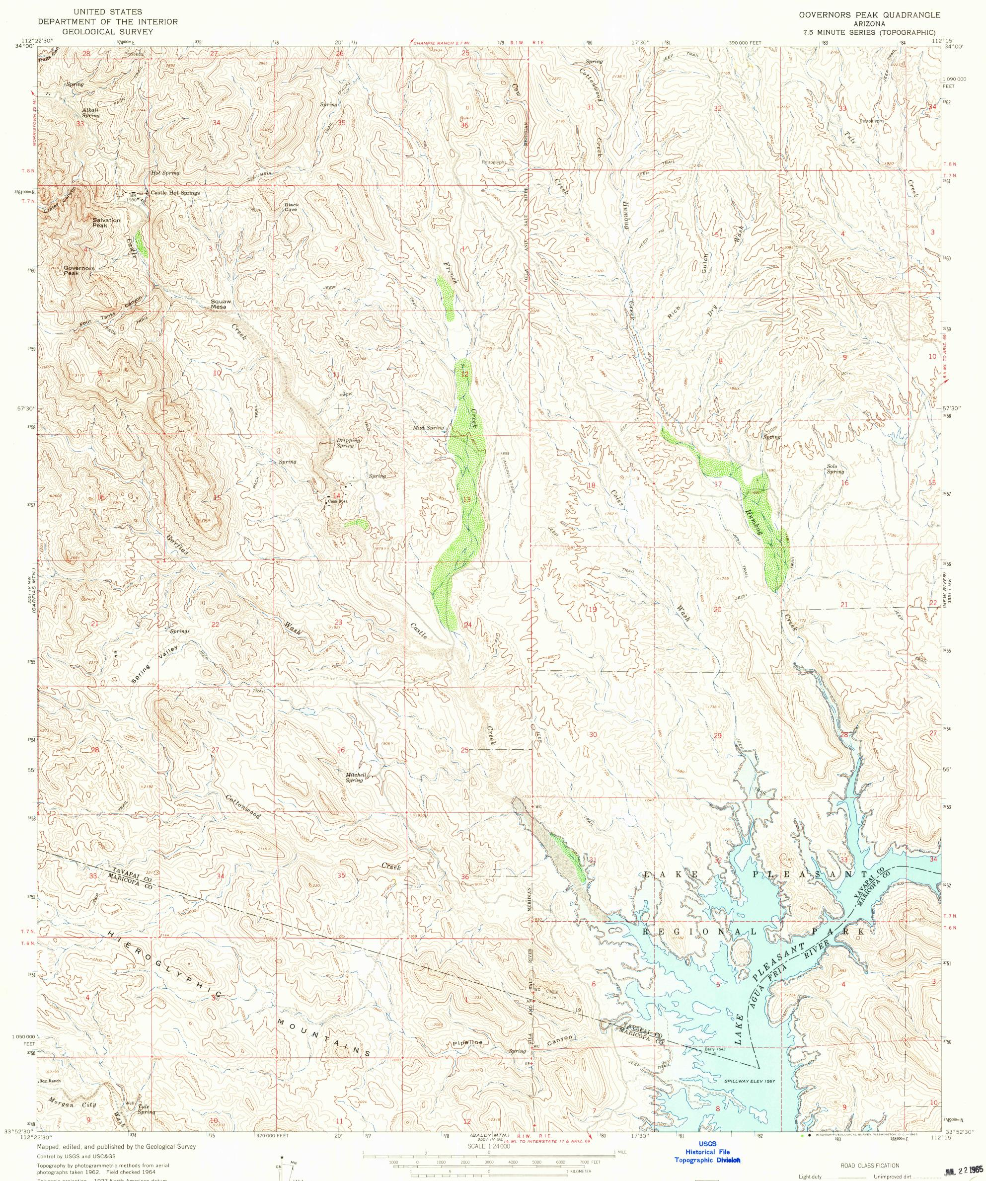
Polyconic projection. 1927 North American datum 10,000-foot grid based on Arizona coordinate system, central zone 1000-meter Universal Transverse Mercator grid ticks, zone 12, shown in blue
