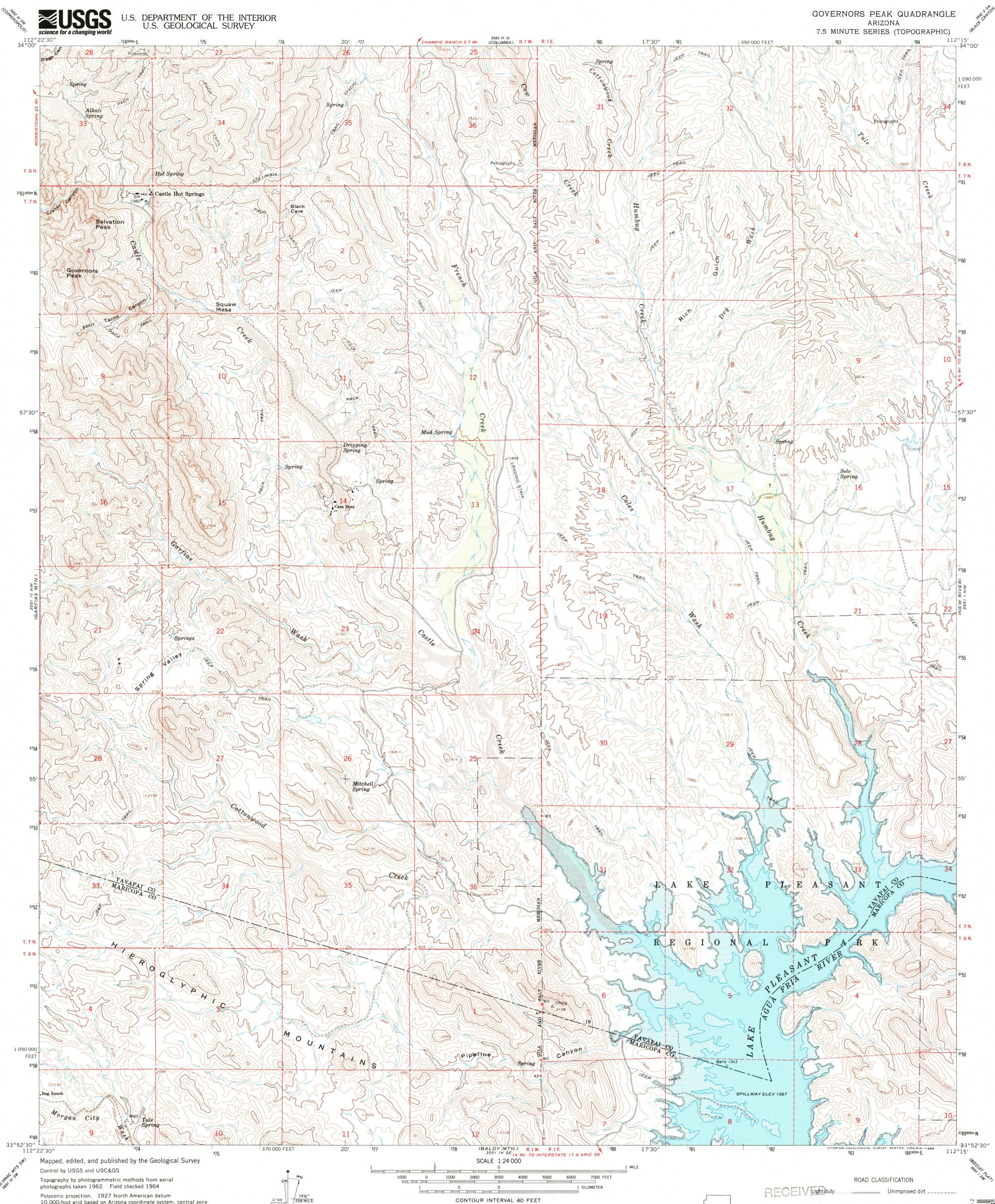
10,000-foot grid based on Arizona coordinate system, central zone 1000-meter Universal Transverse Mercator grid ticks, zone 12, shown in blue To place on the predicted North American Datum 1983 move the projection lines 1 meter south and 66 meters east as shown by dashed corner ticks
