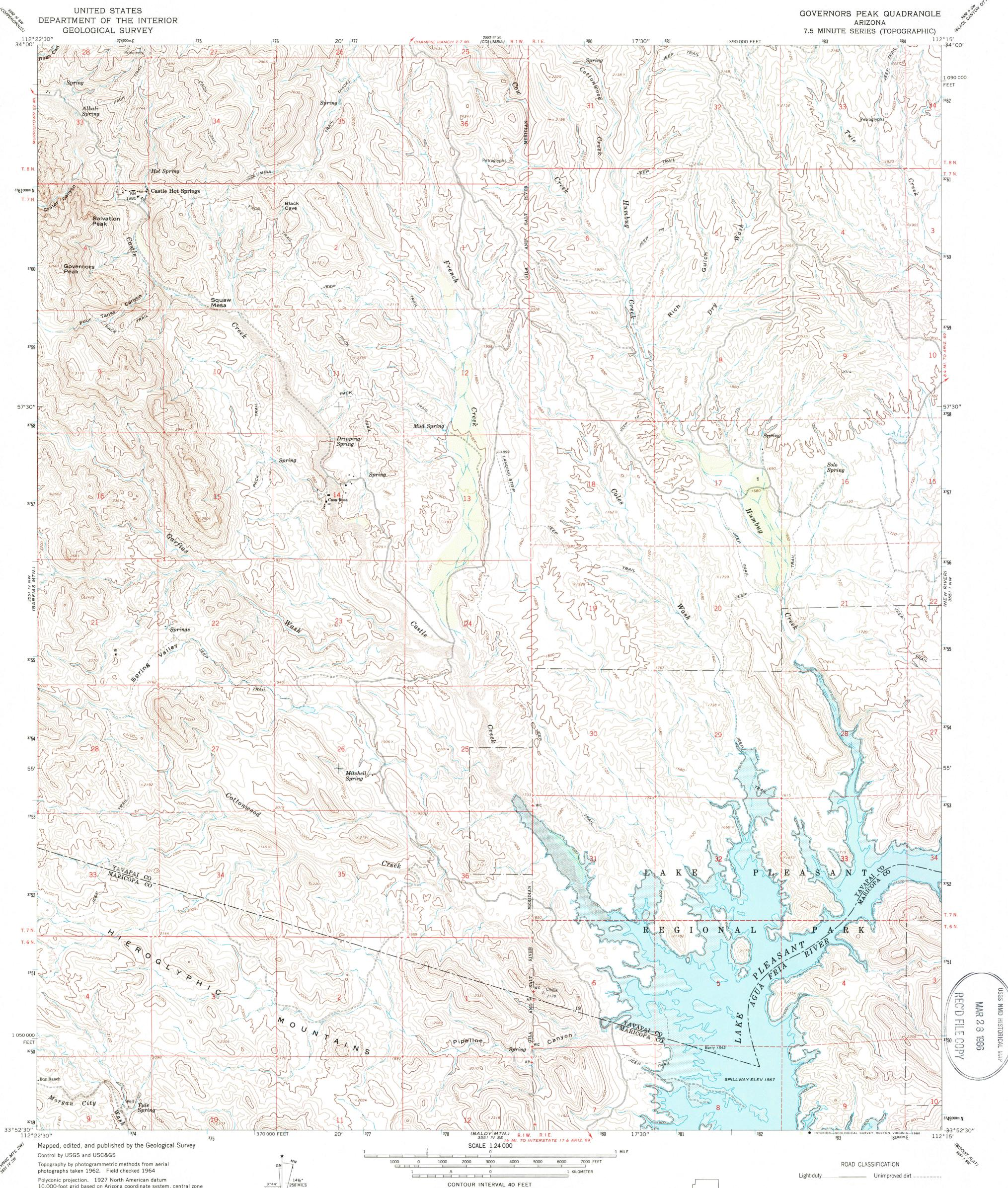
10,000-foot grid based on Arizona coordinate system, central zone 1000-meter Universal Transverse Mercator grid ticks, zone 12, shown in blue To place on the predicted North American Datum 1983 move the projection lines 1 meter south and 66 meters east as shown by dashed corner ticks
