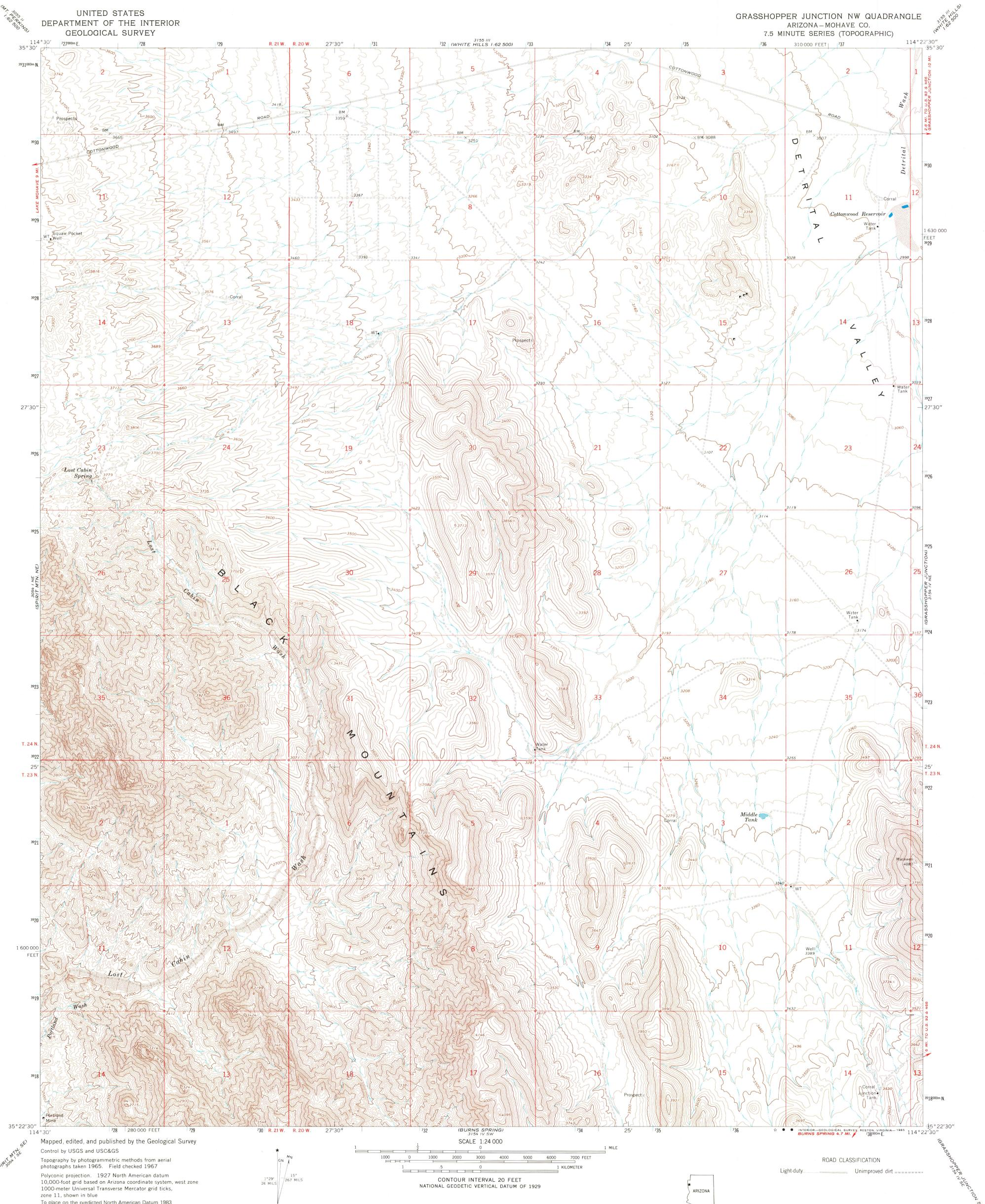
Polyconic projection. 1927 North American datum 10,000-fcot grid based on Arizona coordinate system, west zone 1000-meter Universal Transverse Mercator grid ticks, zone 11, shown in blue To place on the predicted North American Datum 1983 move the projection lines 3 meters north and 73 meters east as shown by dashed corner ticks
