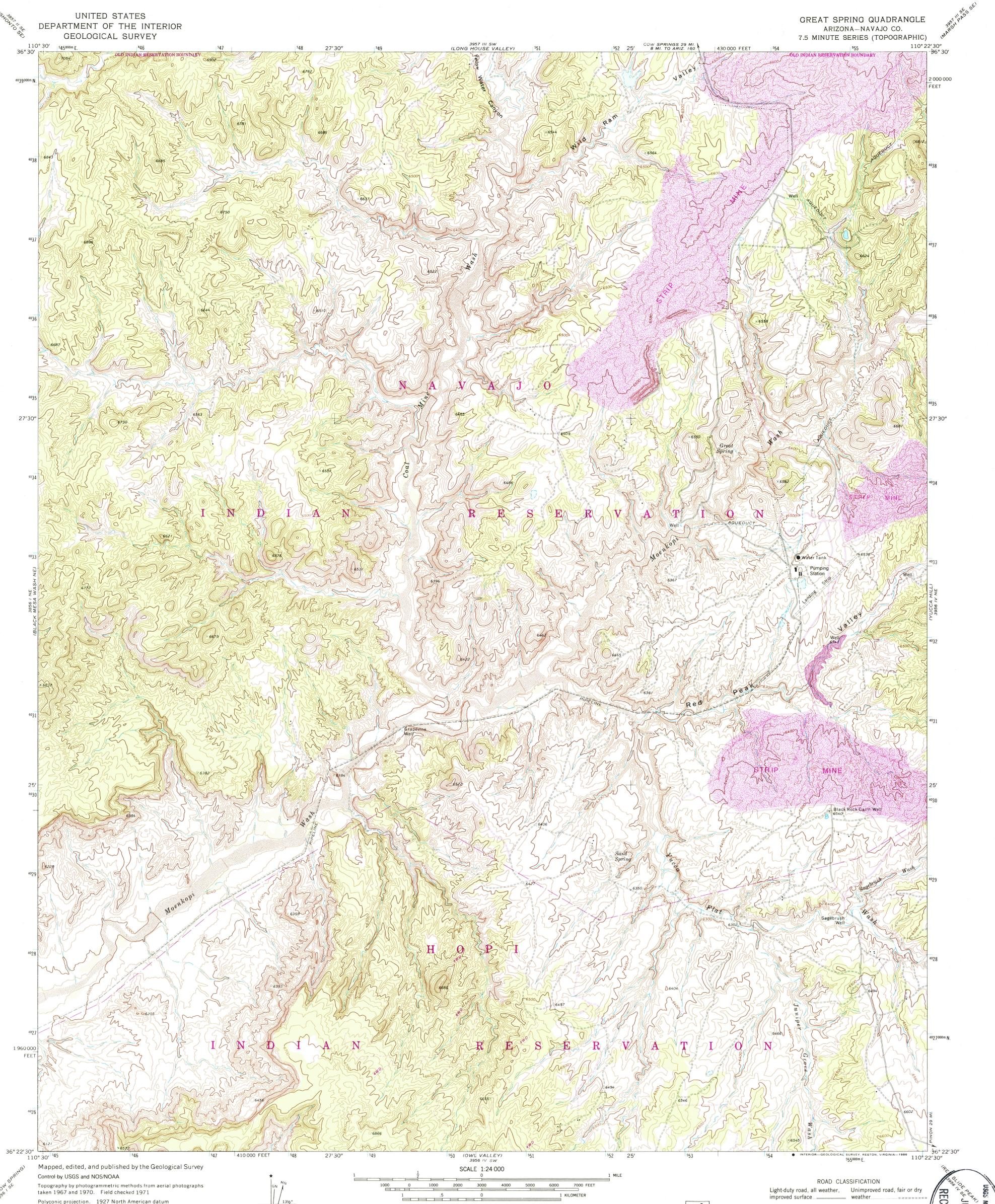
10,000-foot grid based on Arizona coordinate system, east zone 1000-meter Universal Transverse Mercator grid ticks, zone 12, shown in blue To place on the predicted North American Datum 1983 move the projection lines 3 meters north and 62 meters east as shown by dashed corner ticks Land lines have not been established in this area
