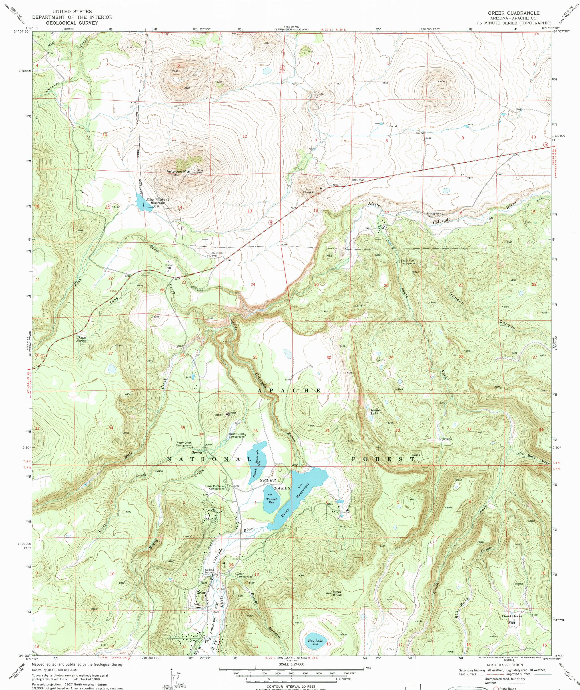
10,000-foot grid based on Arizona coordinate system, east zone 1000-meter Universal Transverse Mercator grid ticks, zone 12, shown in blue To place on the predicted North American Datum 1983
