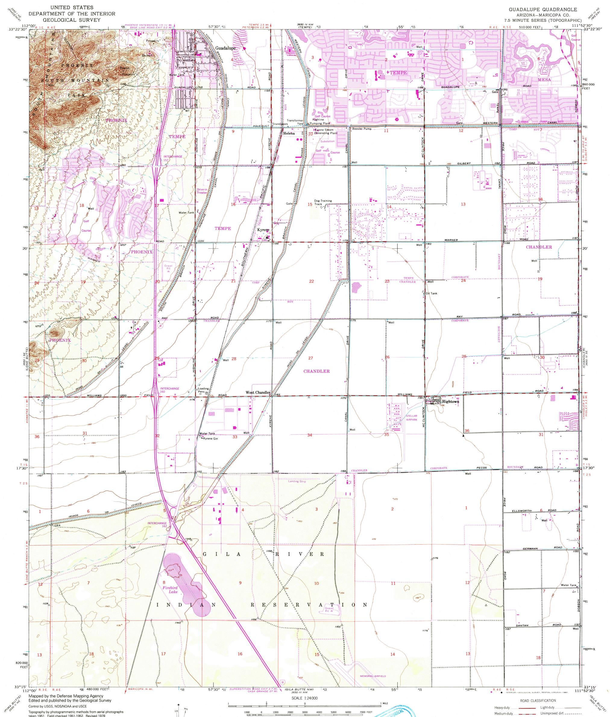
Polyconic projection. 1927 North American Datum 10,000-foot grid based on Arizona coordinate system, central zone 1000-meter Universal Transverse Mercator grid ticks, zone 12, shown in blue The difference between 1927 North American Datum and North American Datum of 1983 (NAD 83) for 7.5 minute intersections is given in USGS Bulletin 1875. The NAD 83 is shown by dashed corner ticks
