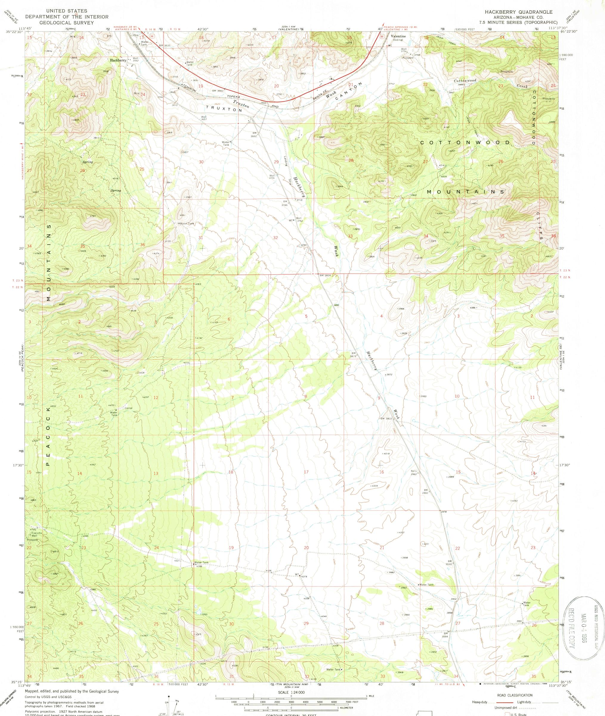
Polyconic projection. 1927 North American datum 10,000-foot grid based on Arizona coordinate system, west zone 1000-meter Universal Transverse Mercator grid ticks, zone 12, shown in blue To place on the predicted North American Datum 1983 move the projection lines 2 meters north and 70 meters east as shown by dashed corner ticks Fine red dashed lines indicate selected fence lines
