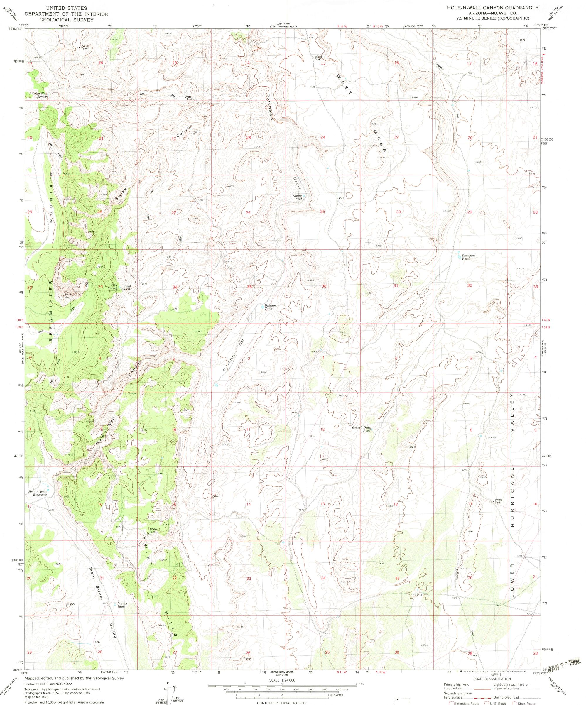
Projection and 10,000-foot grid ticks: Arizona coordinate system, west zone (transverse Mercator) 1000-meter Universal Transverse Mercator grid, zone 12 1927 North American Datum To place on the predicted North American Datum 1983 move the projection lines 5 meters north and 70 meters east as shown by dashed corner ticks
