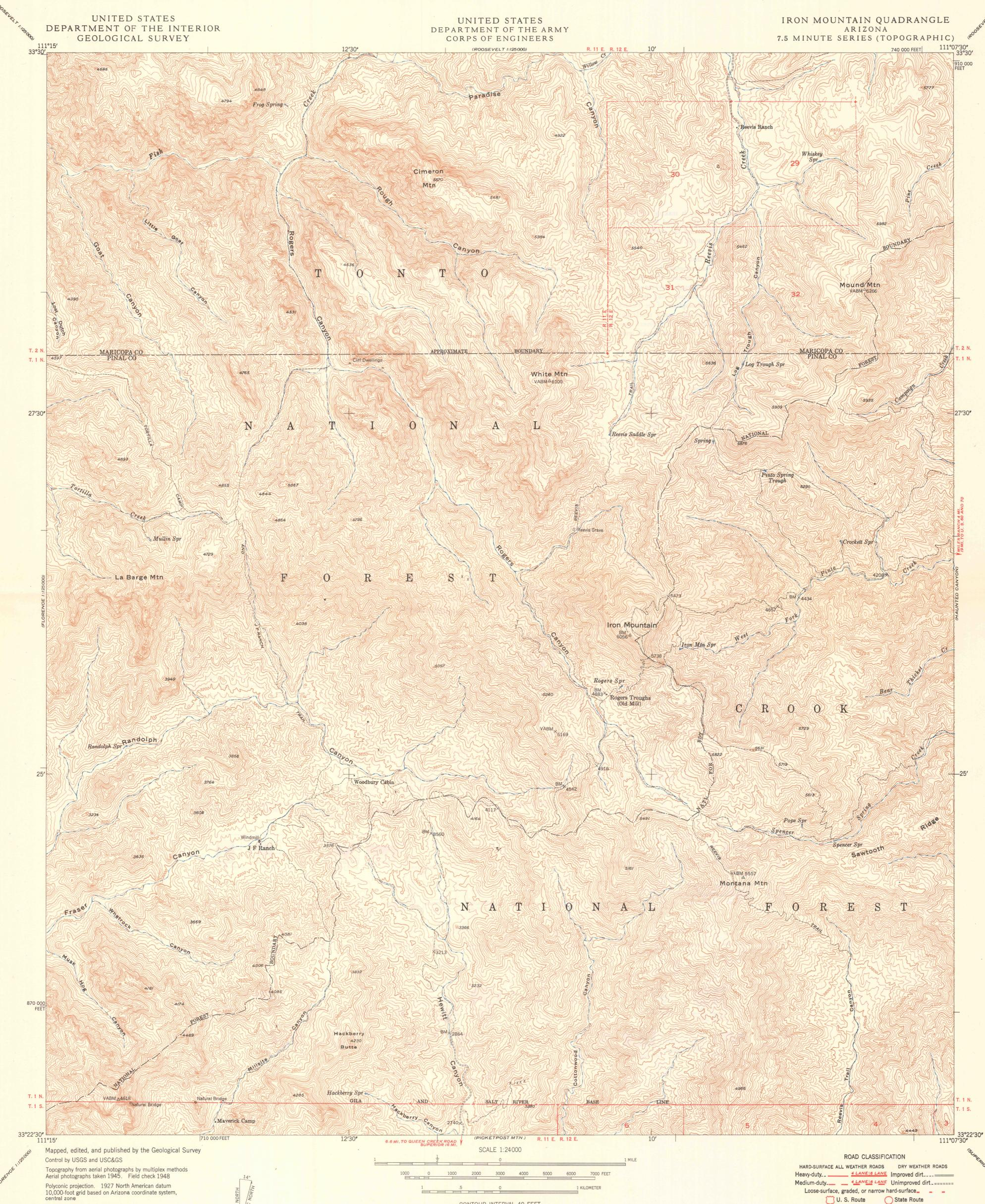
Polyconic projection. 1927 North American datum 10,000-foot grid based on Arizona coordinate system, central zone
