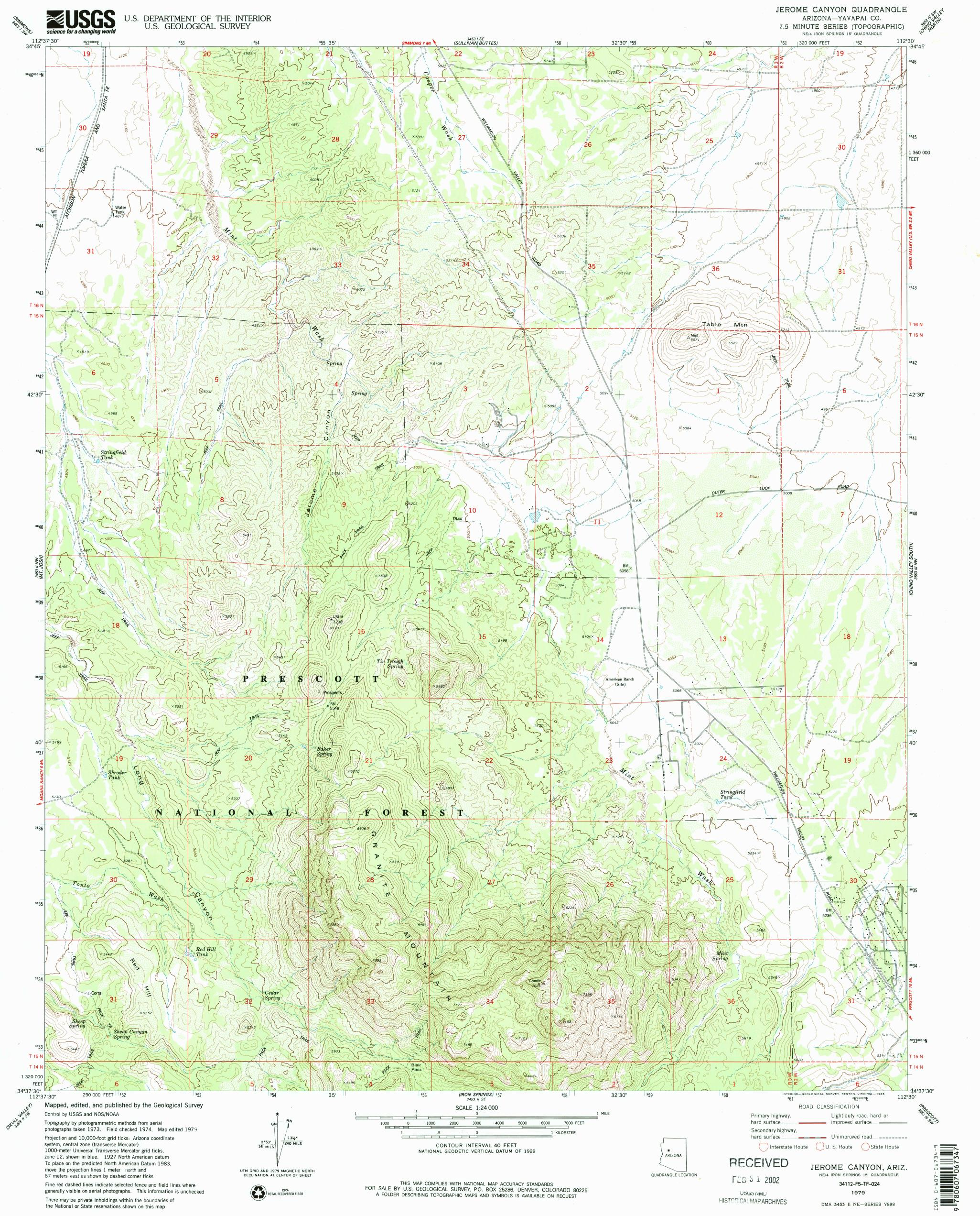
1000-meter Universal Transverse Mercator grid ticks, zone 12, shown in blue. 1927 North American datum To place on the predicted North American Datum 1983, move the projection lines 1 meter north and 67 meters east as shown by dashed corner ticks
