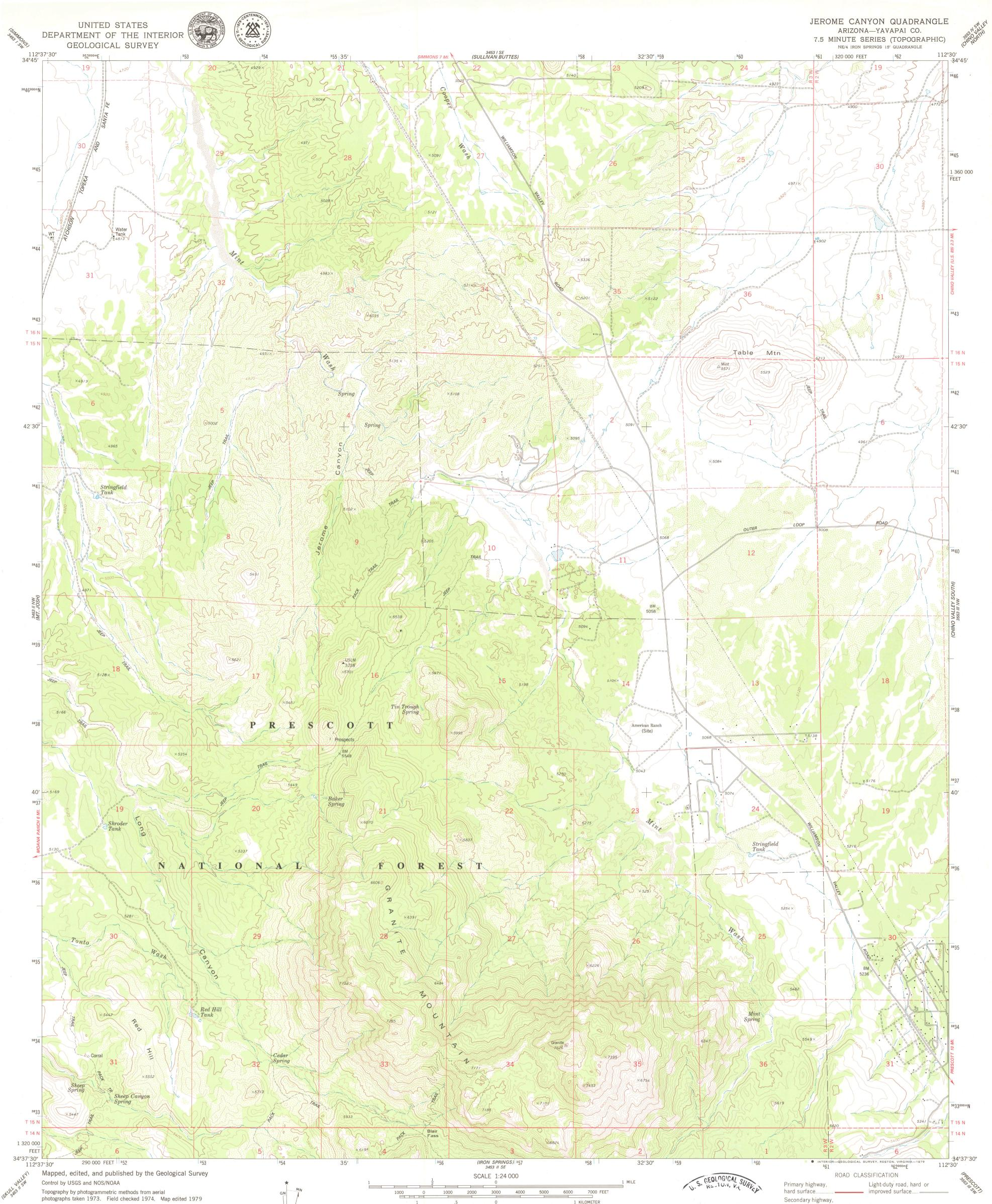
Projection and 10,000-foot grid ticks: Arizona coordinate system, central zone (transverse Mercator) 1000-meter Universal Transverse Mercator grid ticks, zone 12, shown in blue. 1927 North American datum To place on the predicted North American Datum 1983, move the projection lines 1 meters north and 67 meters east as shown by dashed corner ticks
