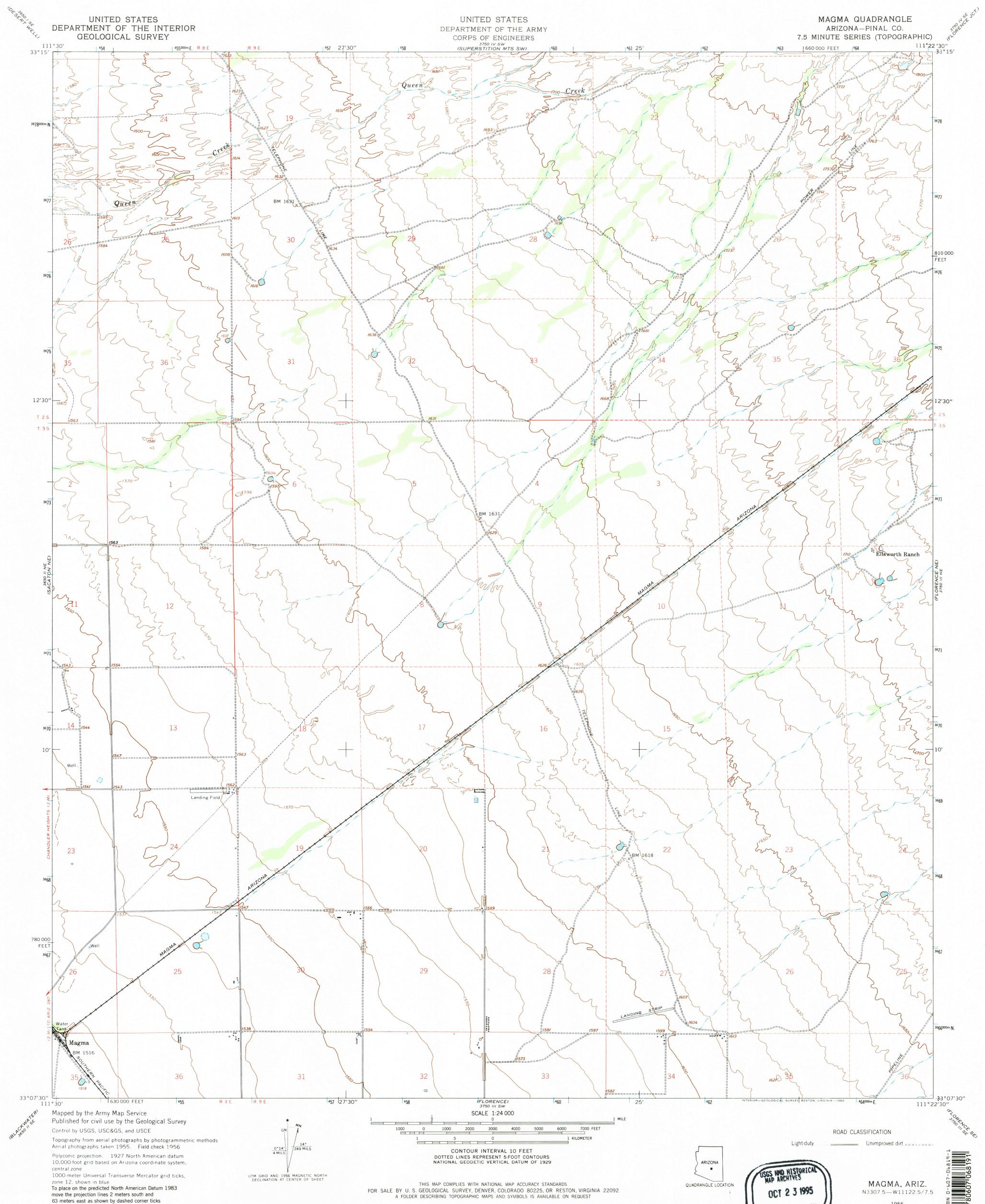
Polyconic projection. 1927 North American datum 10,000-foot grid based on Arizona coordinate system, central zone 1000-meter Universal Transverse Mercator grid ticks, zone 12, shown in blue To place on the predicted North American Datum 1983 move the projection lines 2 meters south and 63 meters east as shown by dashed corner ticks
