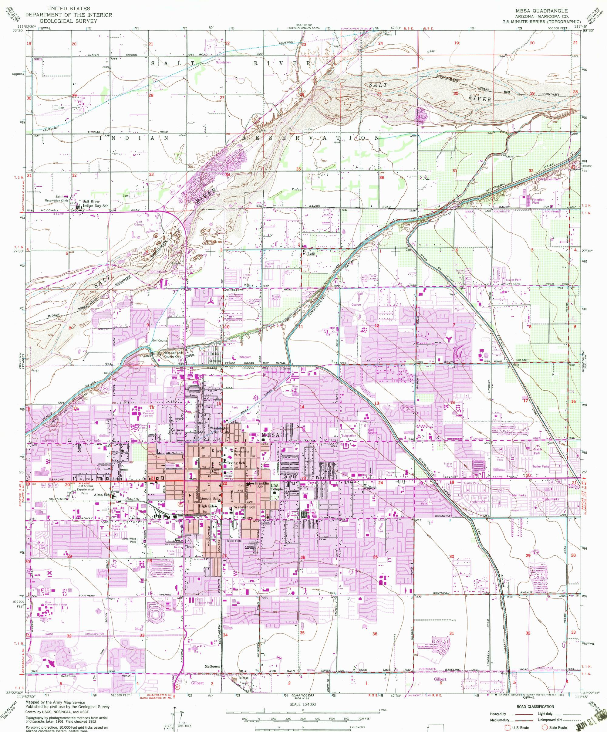
Polyconic projection. 10,000-foot grid ticks based on Arizona coordinate system, central zone 1000-meter Universal Transverse Mercator grid ticks, zone 12, shown in blue. 1927 North American Datum To place on the predicted North American Datum 1983 move the projection lines 2 meters south and 64 meters east as shown by dashed corner ticks
