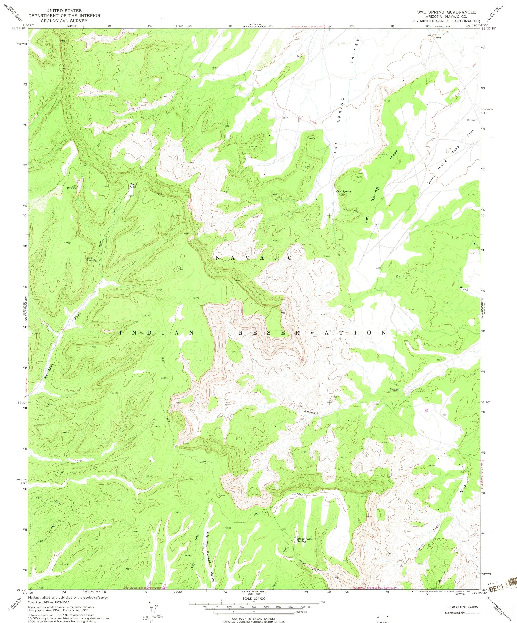
Polyconic projection. 1927 North American datum 10,000-foot grid based on Arizona coordinate system, east zone 1000-meter Universal Transverse Mercator grid ticks, zone 12, shown in blue To place on the predicted North American Datum 1983 move the projection lines 3 meters north and 61 meters east as shown by dashed corner ticks
