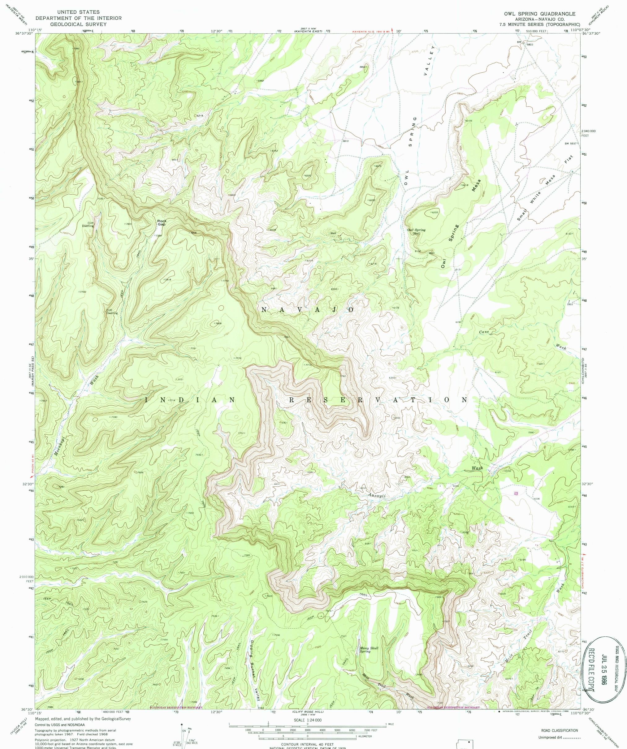
10,000-foot grid based on Arizona coordinate system, east zone 1000-meter Universal Transverse Mercator grid ticks, zone 12, shown in blue To place on the predicted North American Datum 1983 move the projection lines 3 meters north and 61 meters east as shown by dashed corner ticks
