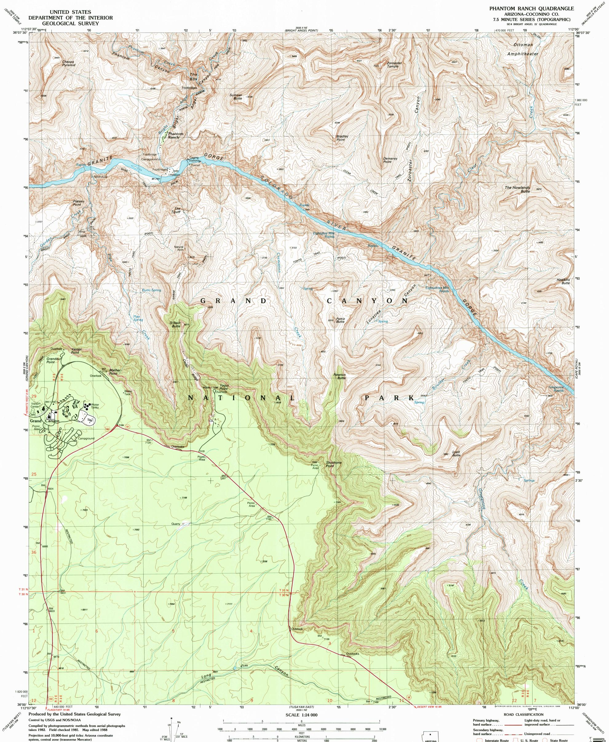
system, central zone (transverse Mercator) 1000-meter Universal Transverse Mercator grid, zone 12 1927 North American Datum To place on the predicted North American Datum 1983 move the projection lines 6 meters north and 66 meters east as shown by dashed corner ticks
