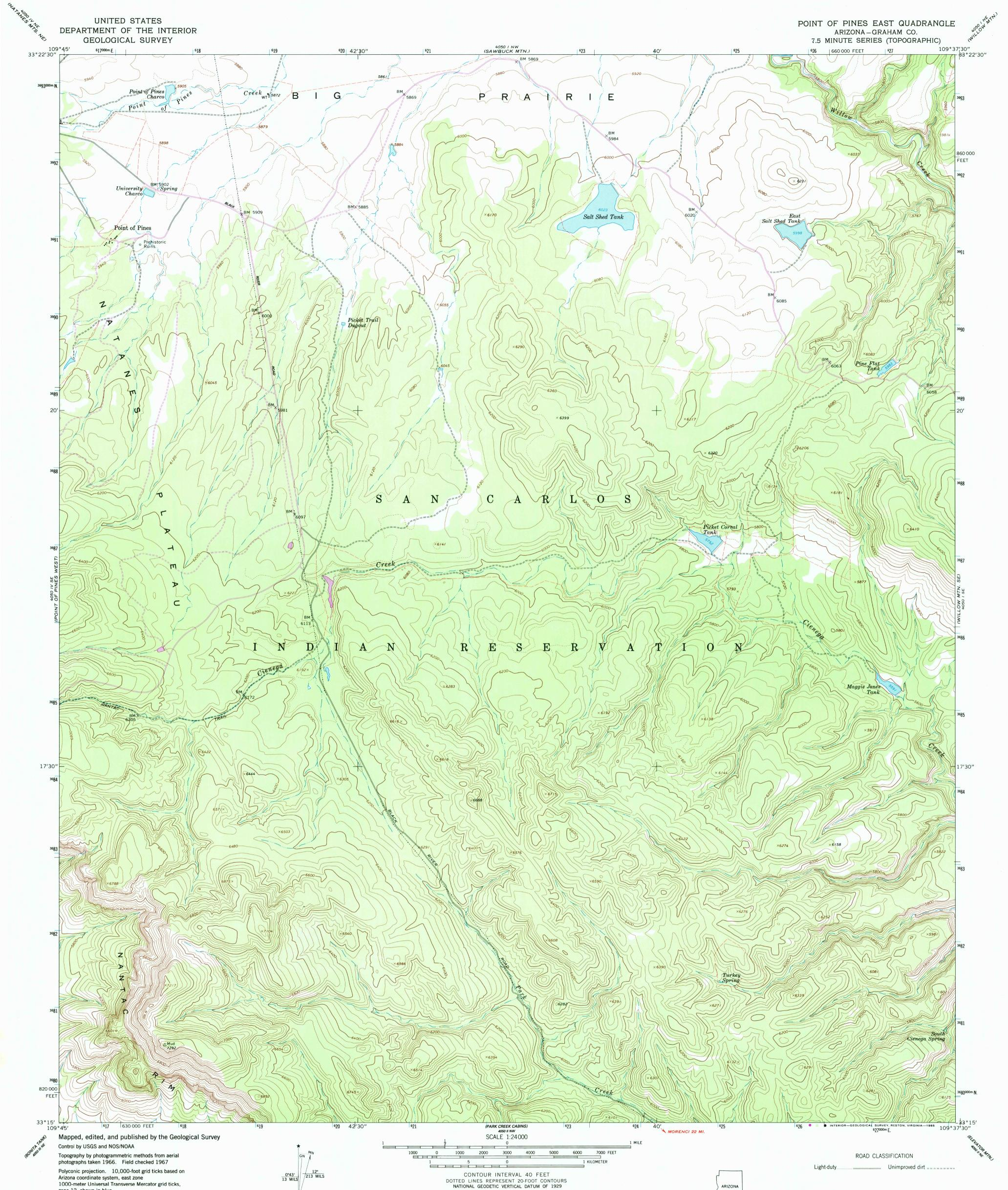
Arizona coordinate system, east zone 1000-meter Universal Transverse Mercator grid ticks, zone 12, shown in blue 1927 North American Datum To place on the predicted North American Datum 1983 move the projection lines 4 meters south and 59 meters east as shown by dashed corner ticks Fine red dashed lines indicate selected fence lines Land lines have not been established in this area
