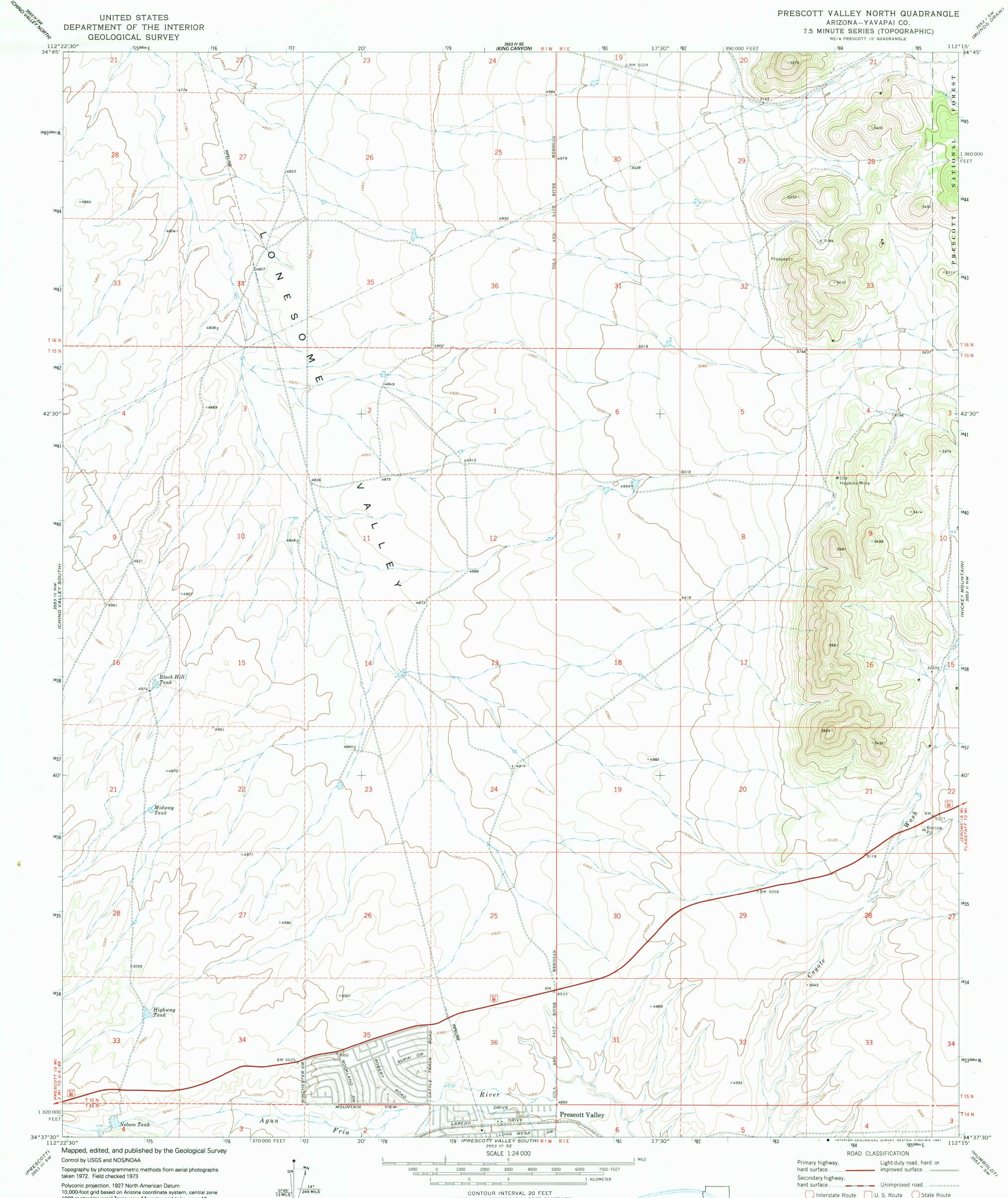
1000-meter Universal Transverse Mercator grid ticks, zone 12 shown in blue. The difference between 1927 North American Datum and North American Datum of 1983 (NAD 83) for 7.5 minute intersections is given in USGS Bulletin 1875. The NAD 83 is shown by dashed corner ticks
