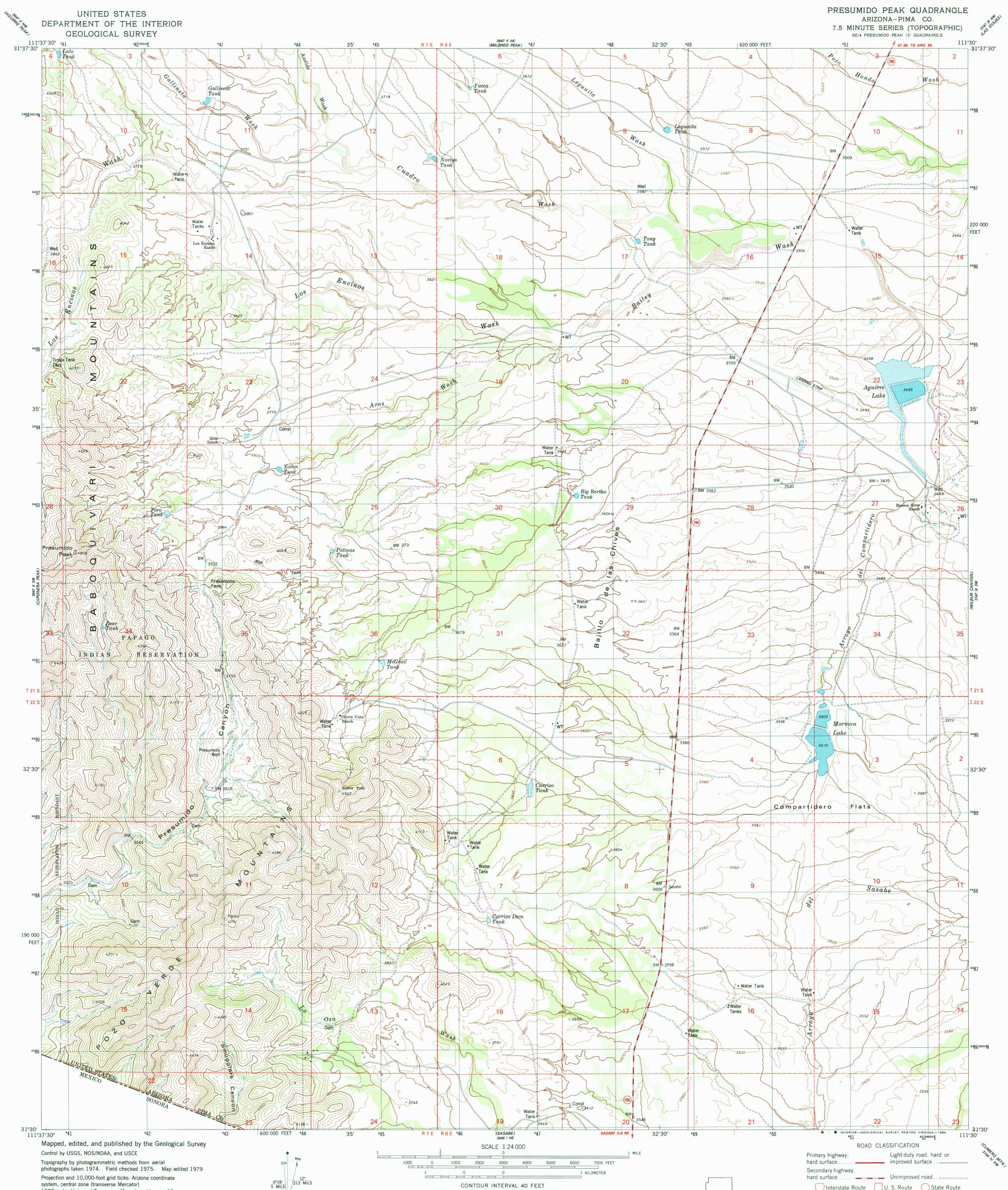
1000-meter Universal Transverse Mercator grid, zone 12 1927 North American Datum To place on the predicted North American Datum 1983 move the projection lines 8 meters south and 64 meters east as shown by dashed corner ticks
