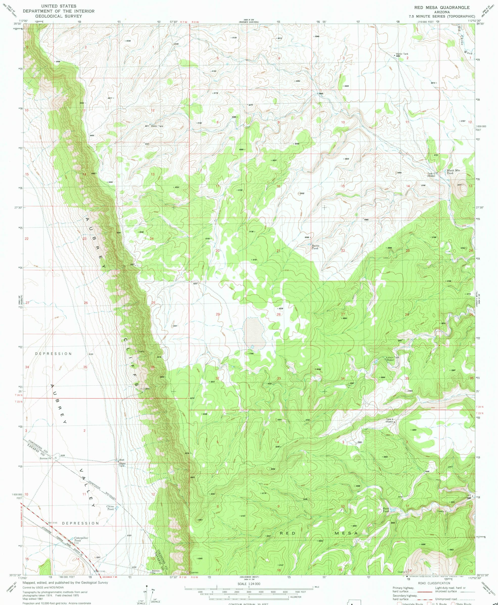
Projection and 10,000-foot grid ticks: Arizona coordinate system, central zone (transverse Mercator) 1000-meter Universal Transverse Mercator grid, zone 12 1927 North American Datum To place on the predicted North American Datum 1983 move the projection lines 3 meters north and 68 meters east as shown by dashed corner ticks
