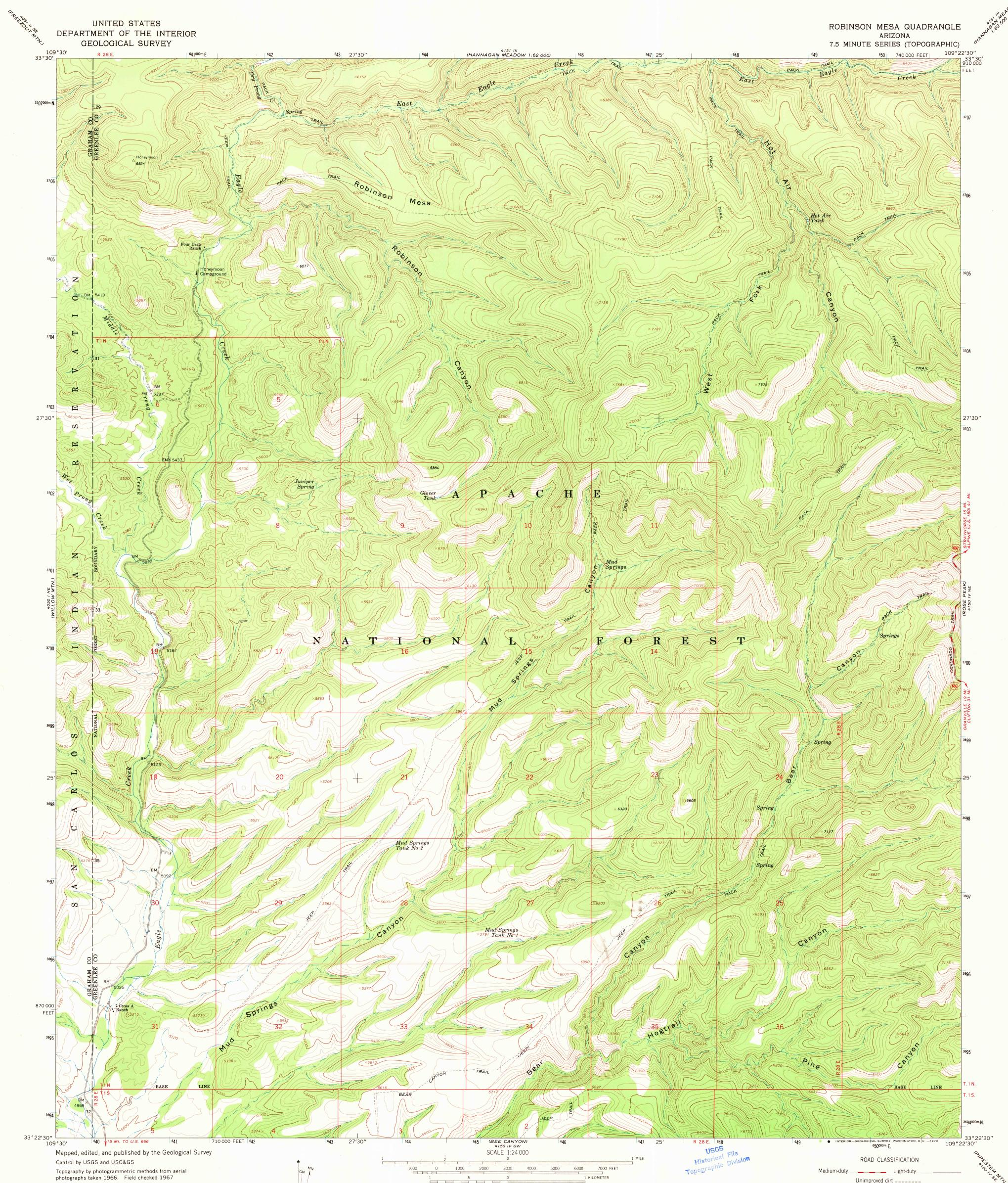
Polyconic projection. 1927 North American datum 10,000-foot grid based on Arizona coordinate system, east zone 1000-meter Universal Transverse Mercator grid ticks, zone 12, shown in blue
