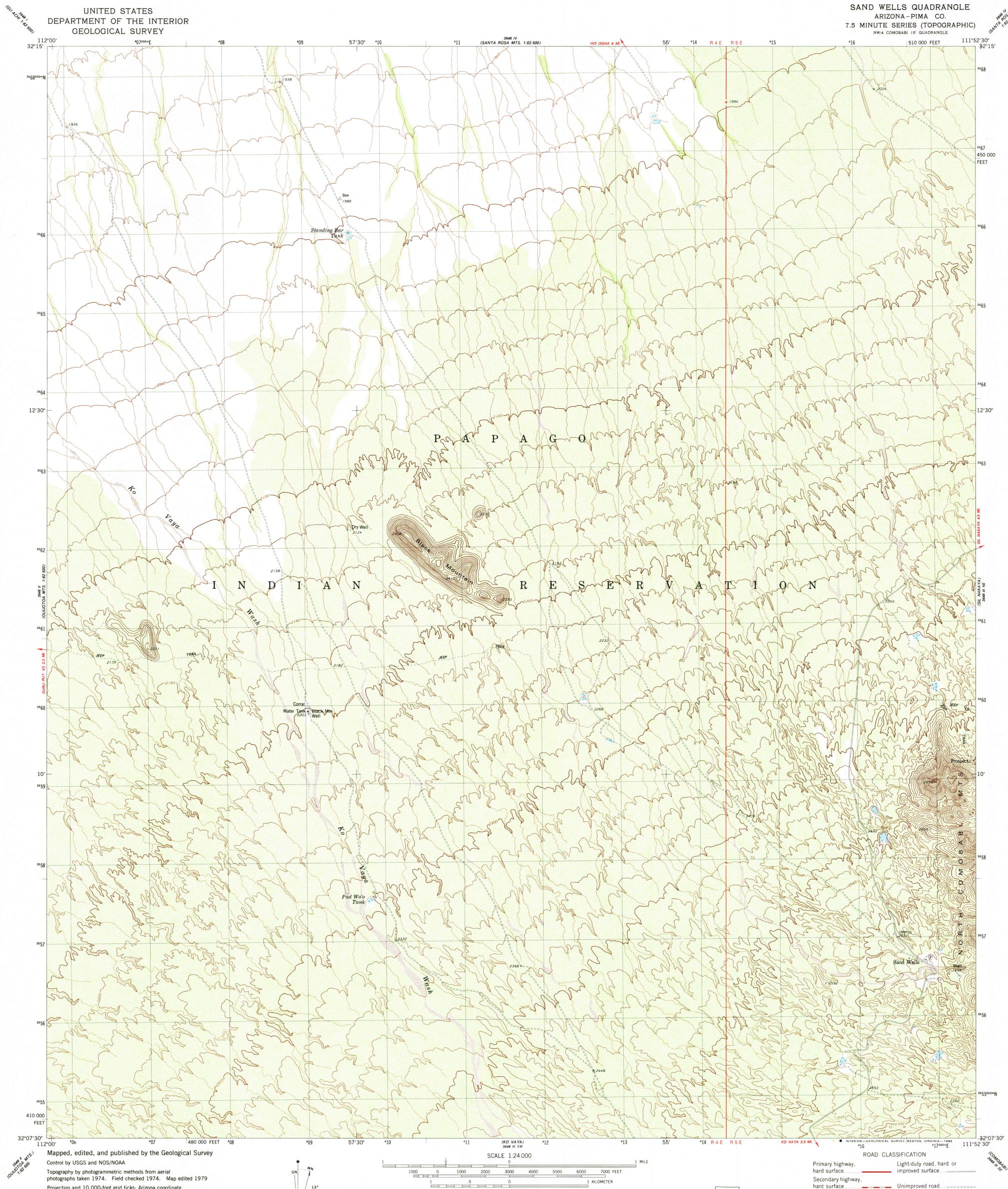
Projection and 10,000-foot grid ticks: Arizona coordinate system, central zone (transverse Mercator) 1000-meter Universal Transverse Mercator grid, zone 12 1927 North American Datum To place on the predicted North American Datum 1983 move the projection lines 5 meters south and 64 meters east as shown by dashed corner ticks
