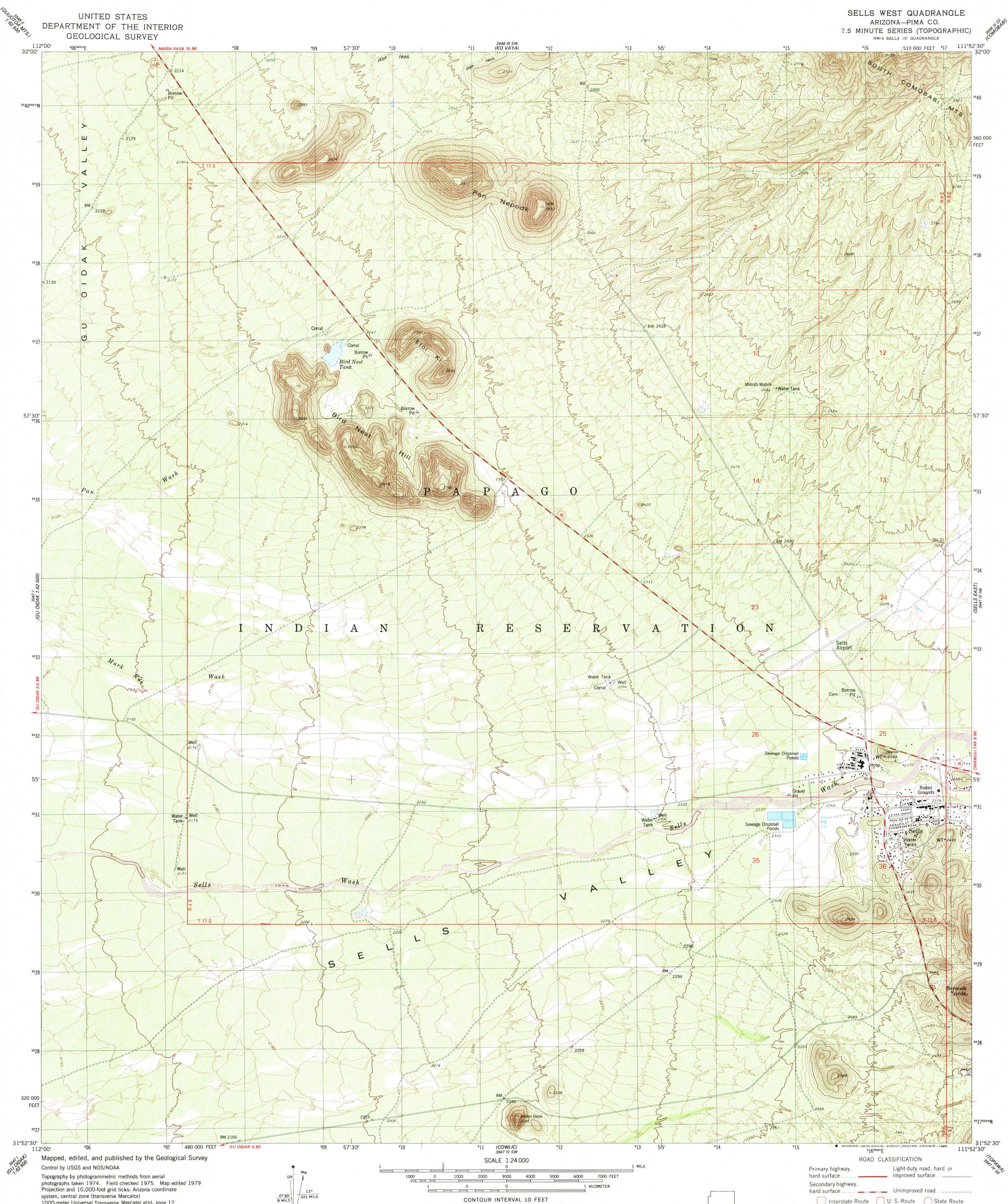
system, central zone (transverse Mercator) 1000-meter Universal Transverse Mercator grid, zone 12 1927 North American Datum To place on the predicted North American Datum 1983 move the projection lines 6 meters south and 64 meters east as shown by dashed corner ticks
