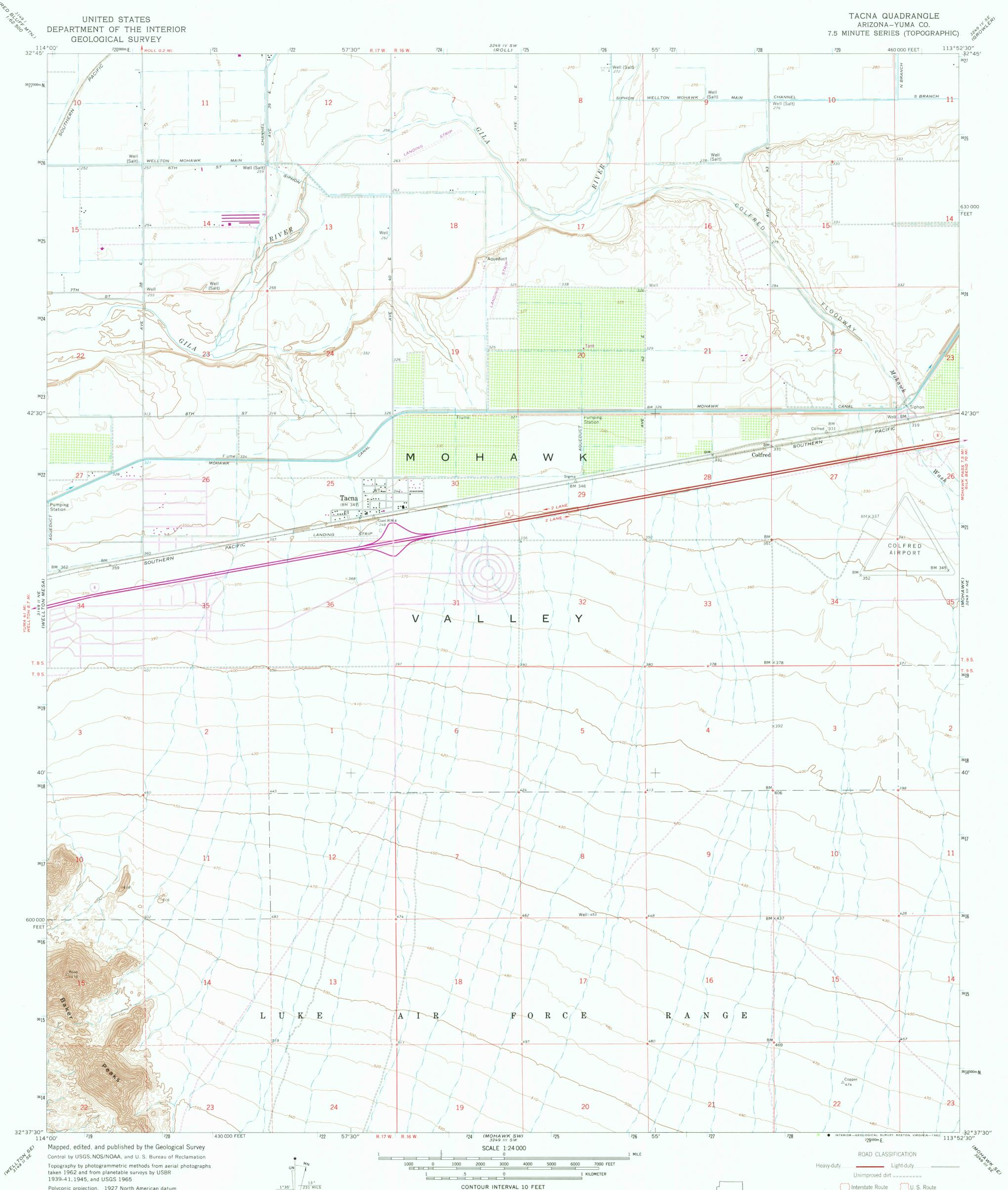
Polyconic projection. 1927 North American datum 10,000-foot grid based on Arizona coordinate system, west zone 1000-meter Universal Transverse Mercator grid ticks, zone 12, shown in blue
