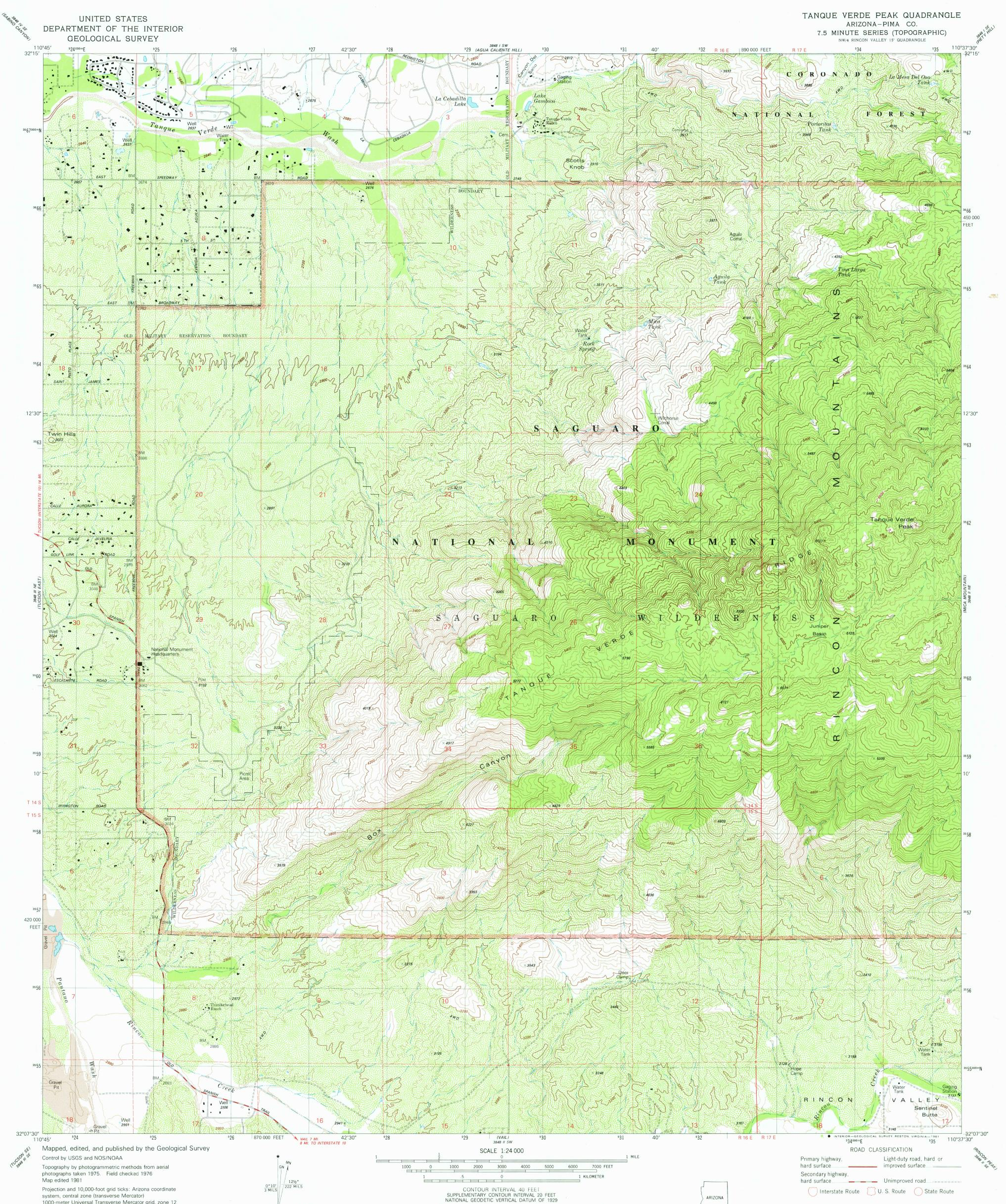
Projection and 10,000-foot grid ticks: Arizona coordinate system, central zone (transverse Mercator) 1000-meter Universal Transverse Mercator grid, zone 12 1927 North American Datum To place on the predicted North American Datum 1983 move the projection lines 6 meters south and 61 meters east as shown by dashed corner ticks Where omitted, land lines have not been established There may be private inholdings within the boundaries of the National or State reservations shown on this map
