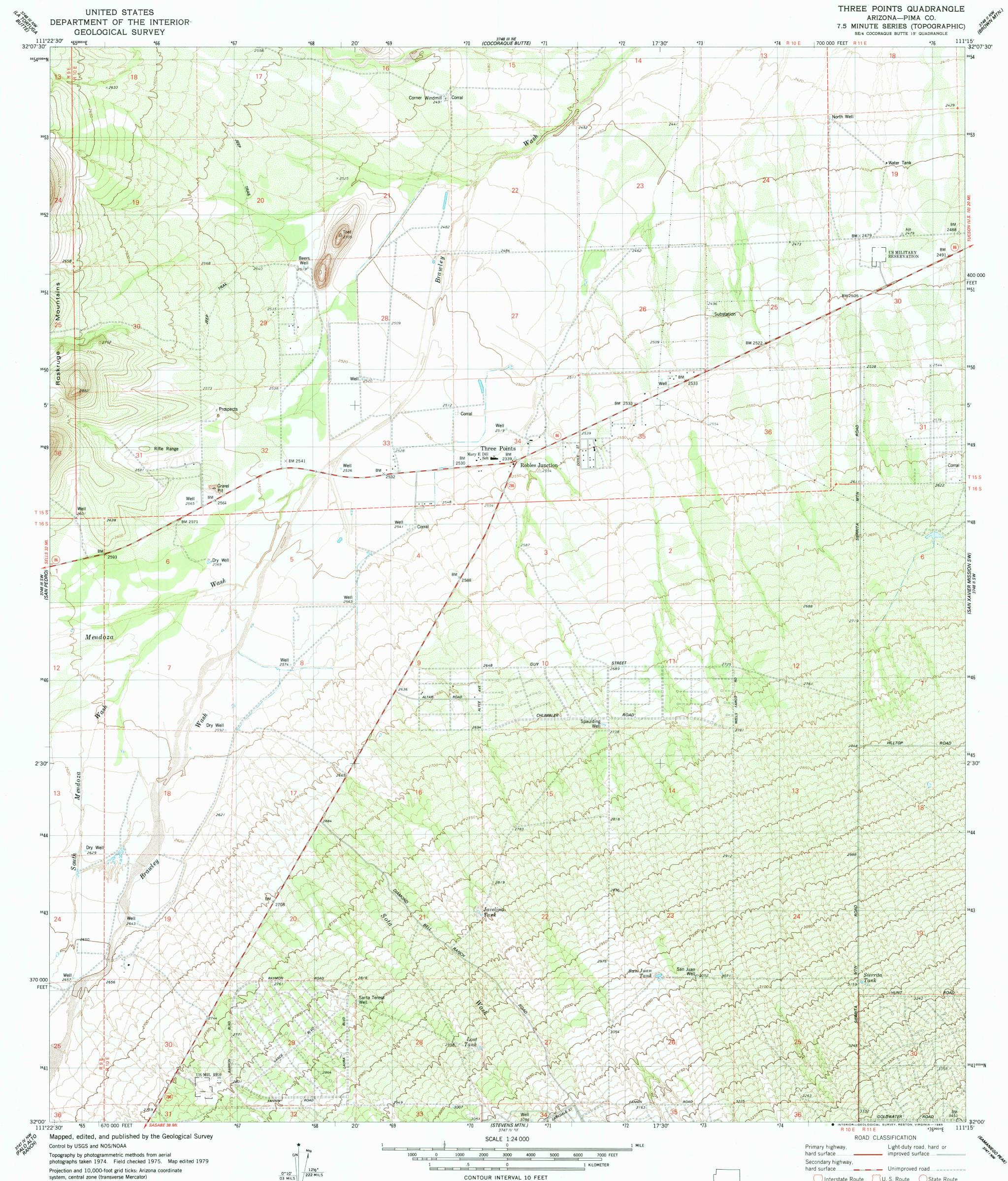
1000-meter Universal Transverse Mercator grid, zone 12 1927 North American Datum To place on the predicted North American Datum 1983 move the projection lines 6 meters south and 63 meters east as shown by dashed corner ticks
