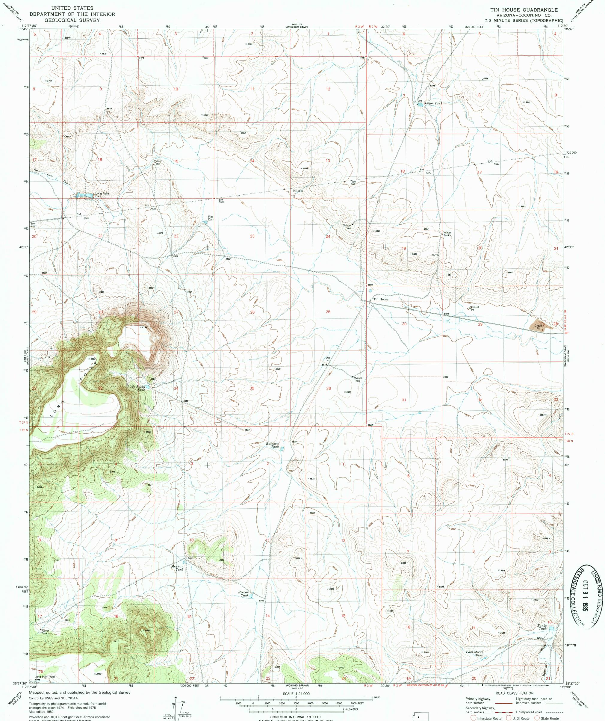
Projection and 10,000-foot grid ticks: Arizona coordinate system, central zone (transverse Mercator) 1000-meter Universal Transverse Mercator grid, zone 12 1927 North American Datum To place on the predicted North American Datum 1983 move the projection lines 4 meters north and 67 meters east as shown by dashed corner ticks
