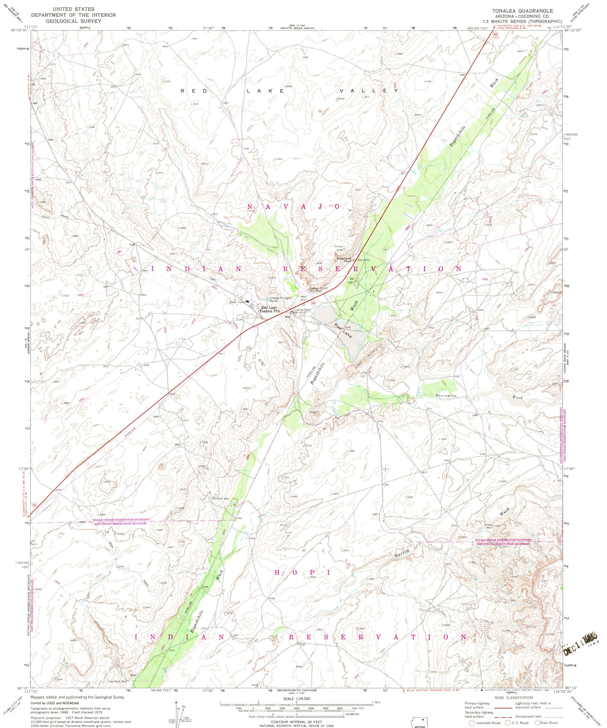
Polyconic projection. 1927 North American datum 10,000-foot grid based on Arizona coordinate system, central zone 1000-meter Universal Transverse Mercator grid ticks, zone 12, shown in blue To place on the predicted North American Datum 1983 move the projection lines 4 meters north and 63 meters east as shown by dashed corner ticks Land lines have not been established in this area There may be private inholdings within the boundaries of the National or State reservations shown on this map
