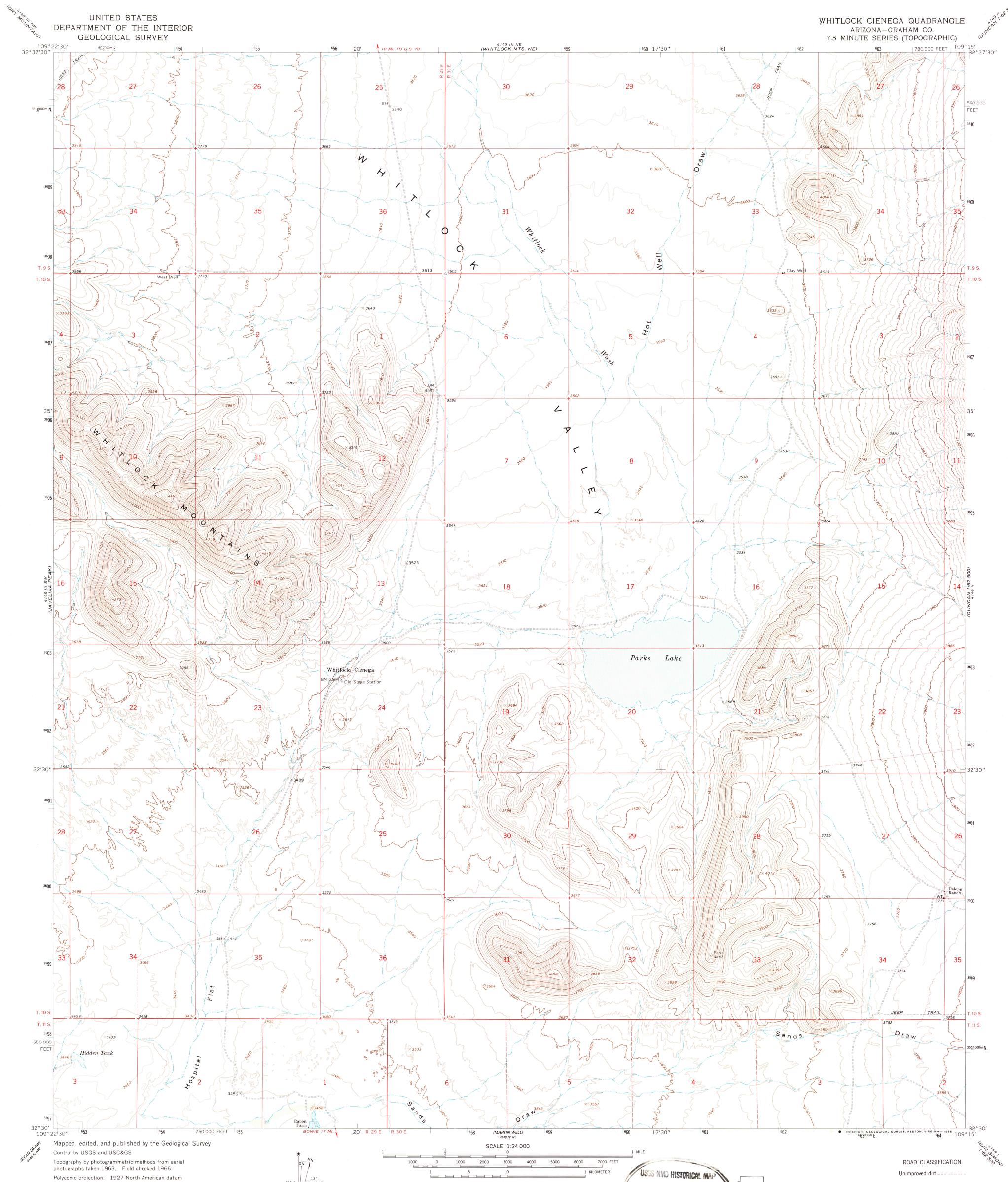
Polyconic projection. 1927 North American datum 10,000-foot grid based on Arizona coordinate system, east zone 1000-meter Universal Transverse Mercator grid ticks, zone 12, shown in blue To place on the predicted North American Datum 1983 move the projection lines 6 meters south and 58 meters east as shown by dashed corner ticks Fine red dashed lines indicate selected fence lines
