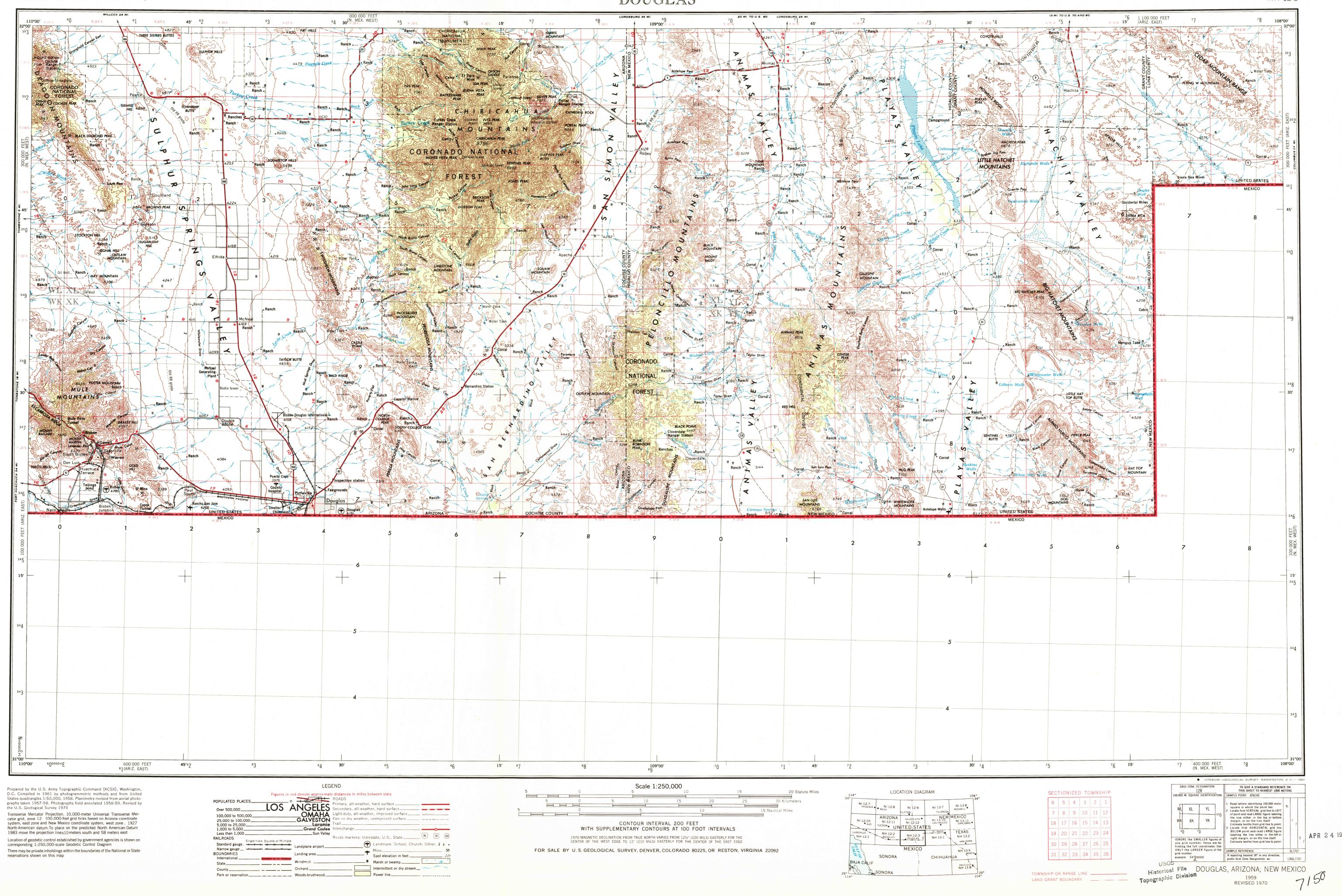
Transverse Mercator Projection. 10,000-meter Universal Transverse Mer-cator grid, zone 12. 100,000-foot grid ticks based on Arizona coordinate system, east zone and New Mexico coordinate system, west zone . 1927 North American datum. To place on the predicted North American Datum 1983 move the projection lines10 meters south and 58 meters east
