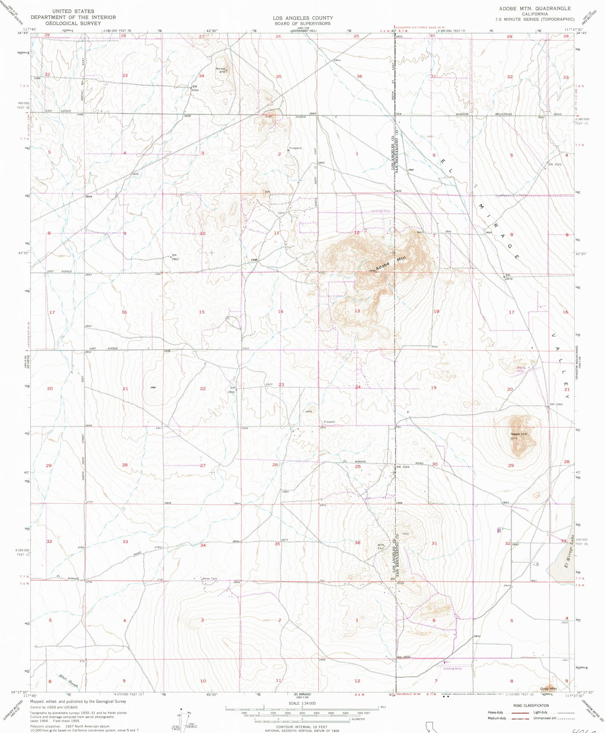
Polyconic projection. 1927 North American datum 10,000-foot grids based on California coordinate system, zones 5 and 7 1000-meter Universal Transverse Mercator grid ticks, zone 11, shown in blue
