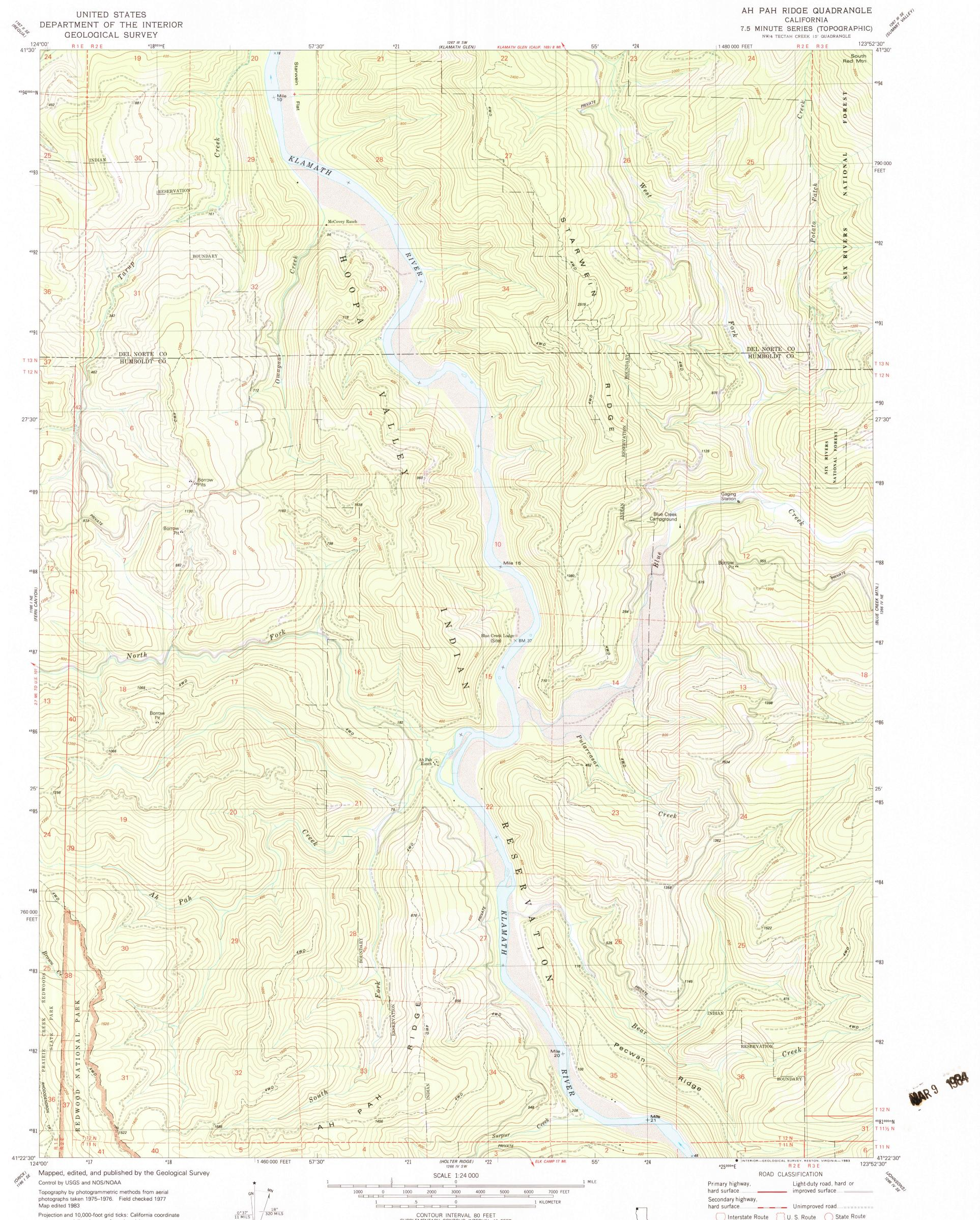
system, zone 1 (Lambert conformal conic) 1000-meter Universal Transverse Mercator grid, zone 10 1927 North American Datum UTM GRID AND 1983 MAGNETIC NORTH DECLINATION AT CENTER OF SHEET To place on the predicted North American Datum 1983 move the projection lines 21 meters north and 97 meters east as shown by dashed corner ticks Certain land lines are omitted because of insufficient data There may be private inholdings within the boundaries of the National or State reservations shown on this map
