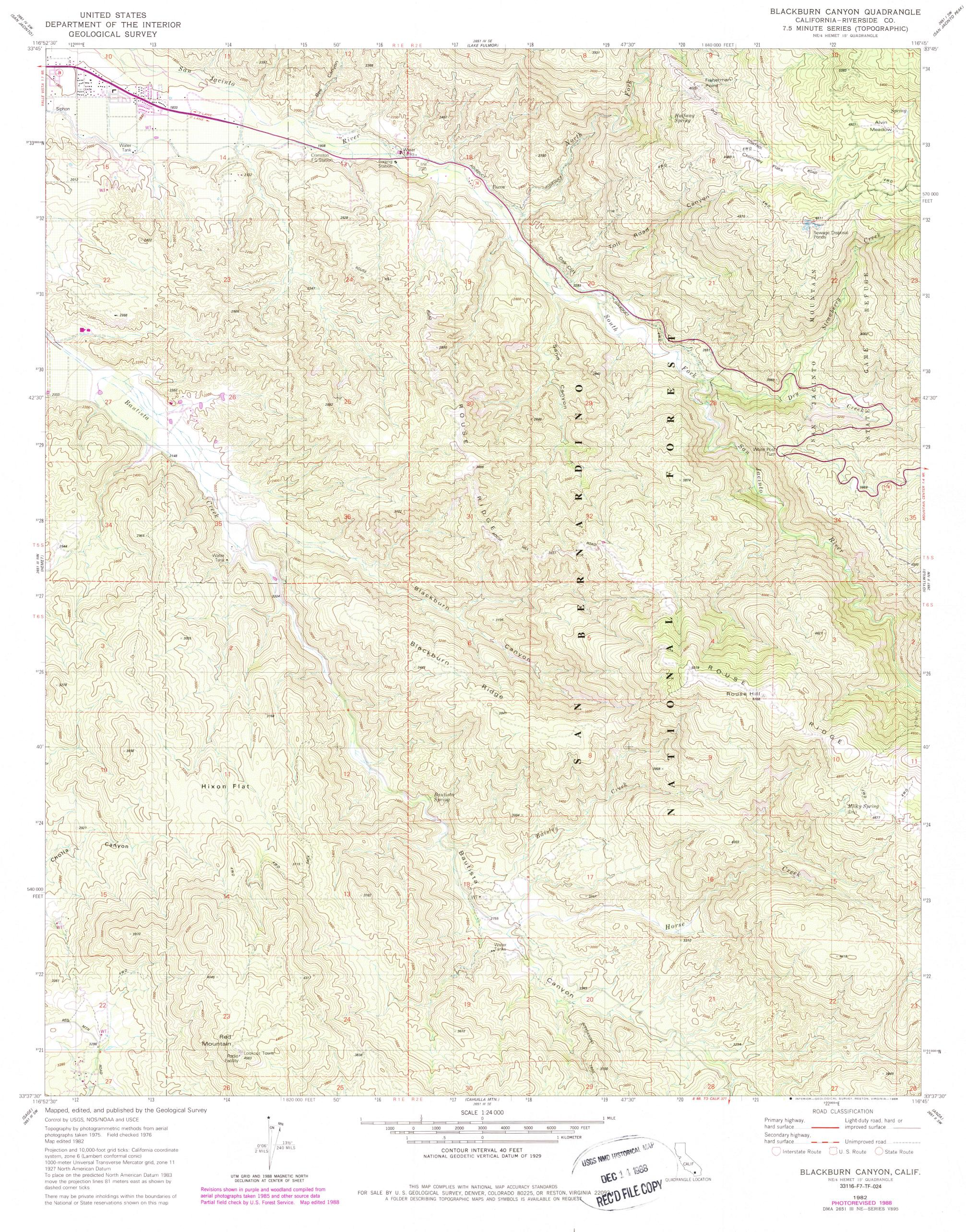
Projection and 10,000-foot grid ticks: California coordinate system, zone 6 (Lambert conformal conic) 1000-meter Universal Transverse Mercator grid, zone 11 1927 North American Datum To place on the predicted North American Datum 1983 move the projection lines 81 meters east as shown by dashed corner ticks
