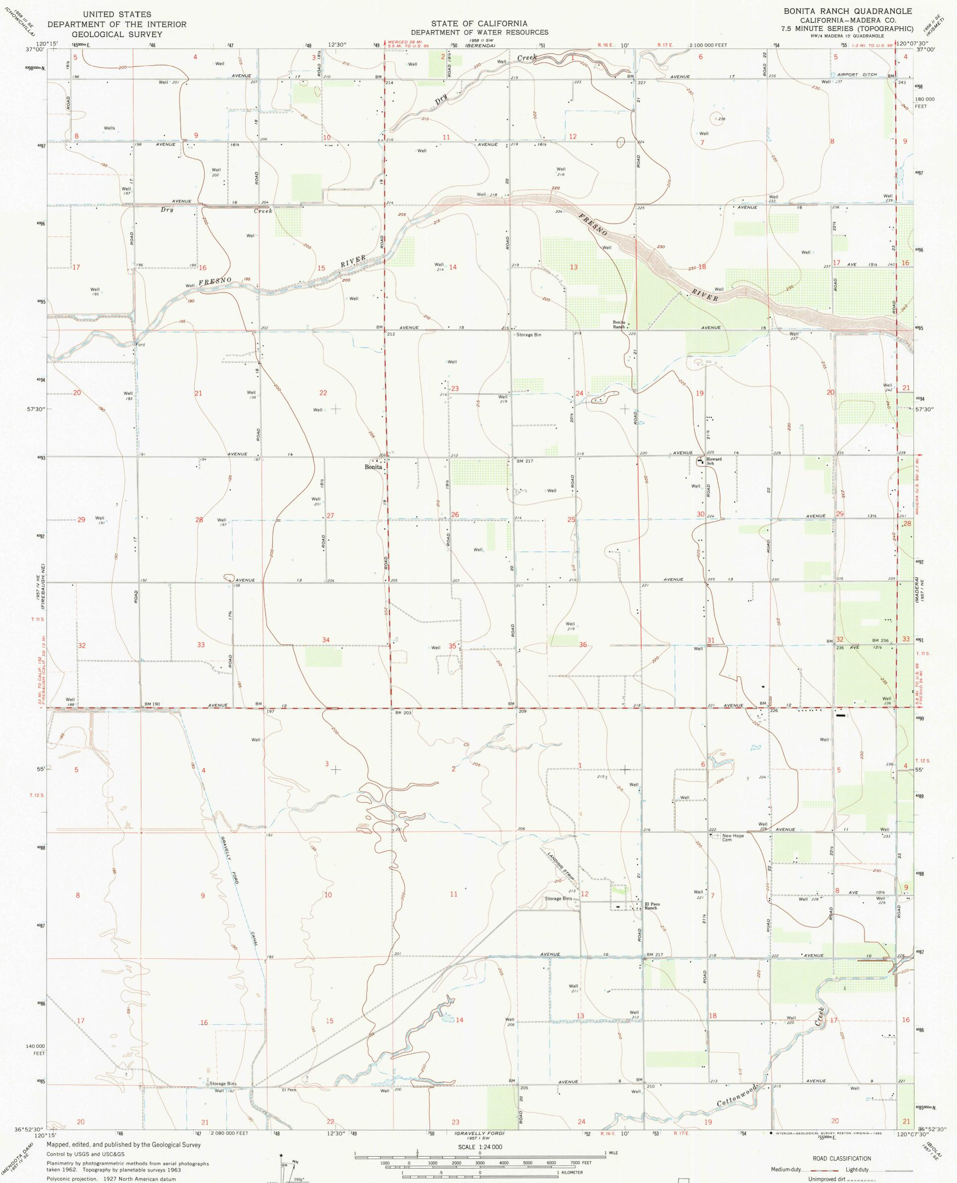
10,000-foot grid based on California coordinate system, zone 3 1000-meter Universal Transverse Mercator grid ticks, zone 10, shown in blue To place on the predicted North American Datum 1983 move the projection lines 9 meters north and 89 meters east as shown by dashed corner ticks Fine red dashed lines indicate selected fence lines A portion of the south half of this map lies within a subsidence area Vertical control based on latest available adjustment
