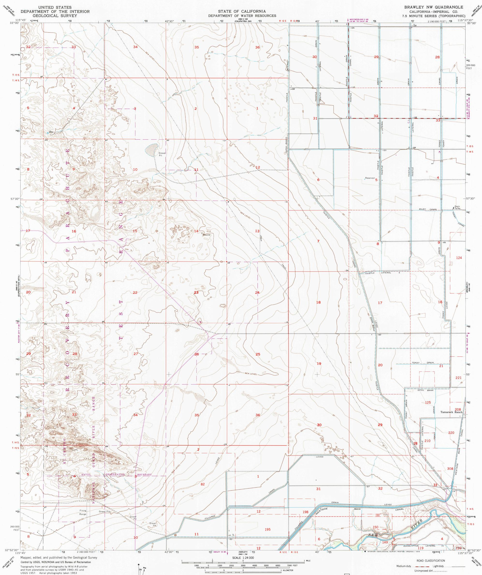
Polyconic projection. 1927 North American datum 10,000-foot grid based on California coordinate system, zone 6 1000-meter Universal Transverse Mercator grid ticks, zone 11, shown in blue To place on the predicted North American Datum 1983 move the projection lines 4 meters south and 76 meters east as shown by dashed corner ticks
