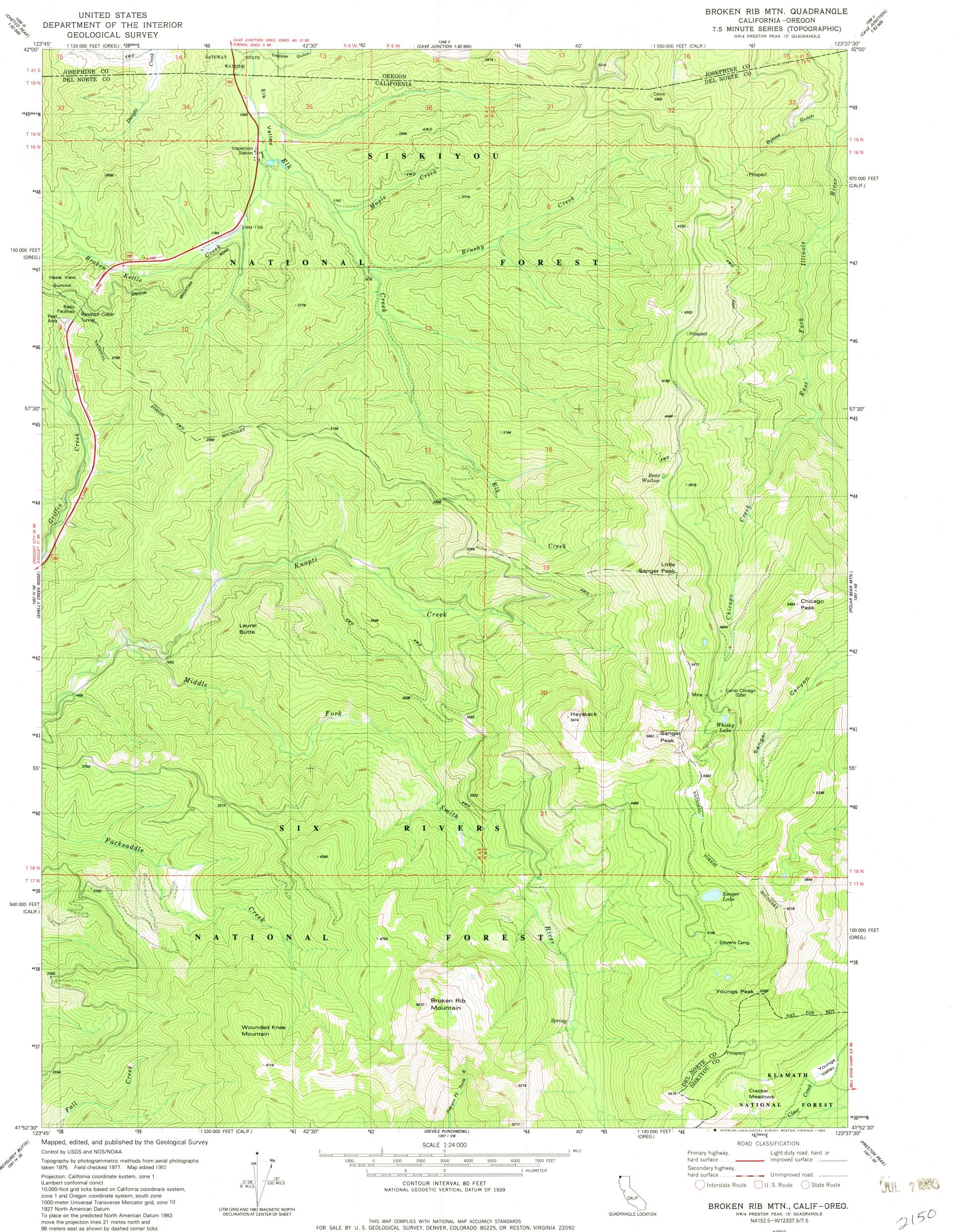
(Lambert conformal conic) 10,000-foot grid ticks based on California coordinate system, zone 1 and Oregon coordinate system, south zone 1000-meter Universal Transverse Mercator grid, zone 10 1927 North American Datum To place on the predicted North American Datum 1983 move the projection lines 21 metes north and 96 meters east as shown by dashed corner ticks Certain land lines are omitted because of insufficient data
