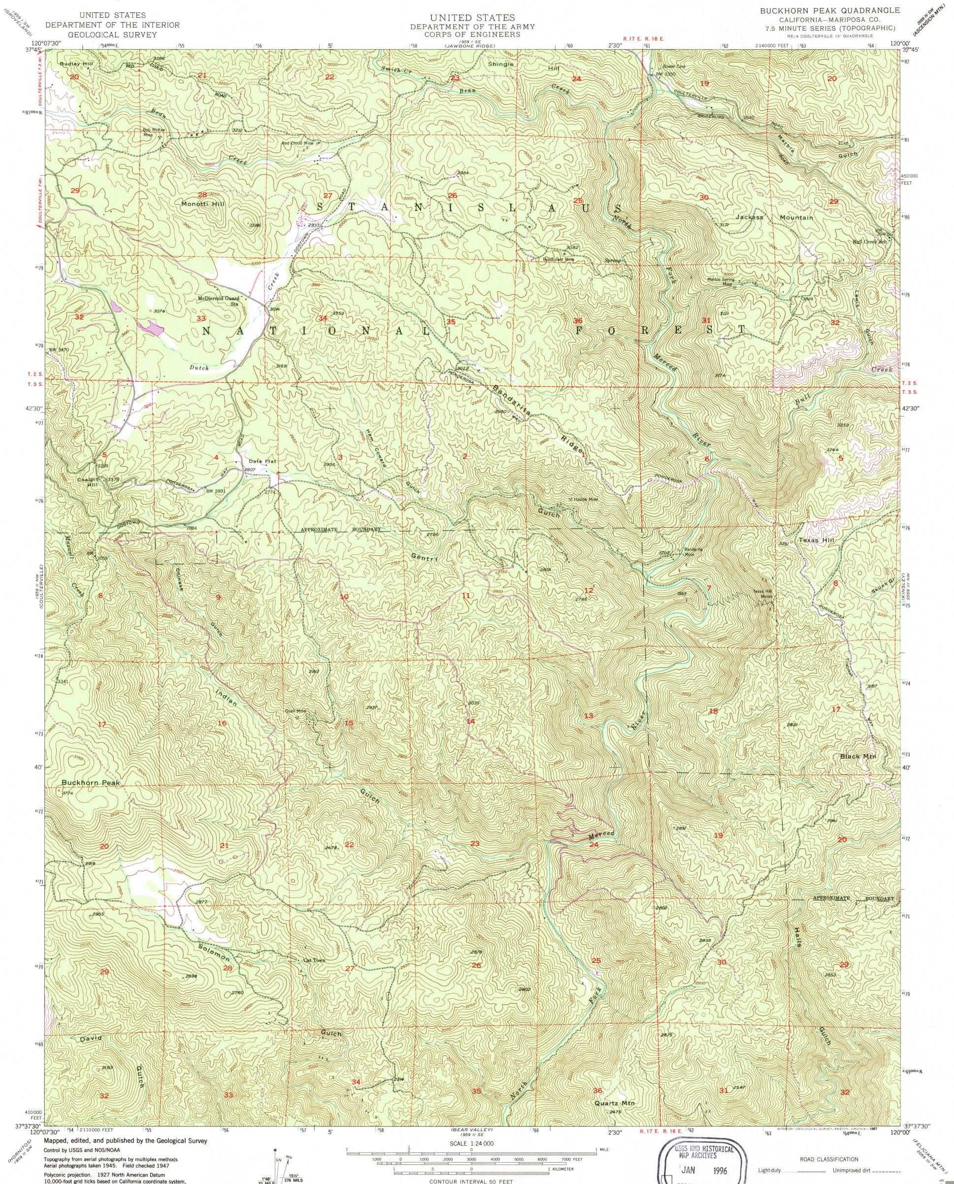
10,000-foot grid ticks based on California coordinate system, zone 3 1000-meter Universal Transverse Mercator grid ticks, zone 10, shown in blue To place on the predicted North American Datum 1983, move the projection lines 11 meters north and 88 meters east as shown by dashed corner ticks
