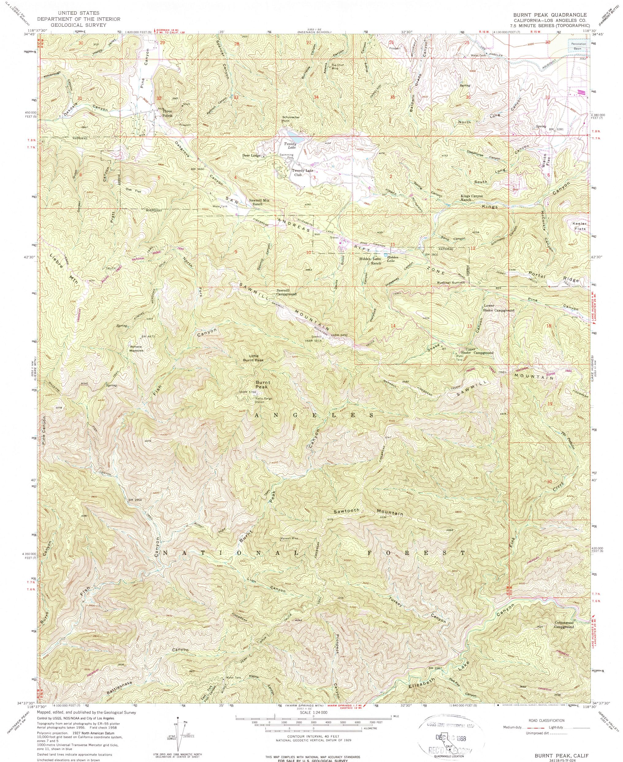
To place on the predicted North American Datum 1983 move the projection lines 5 meters north and 85 meters east as shown by dashed corner ticks Previous revisions compiled in cooperation with California Department of Water Resources
