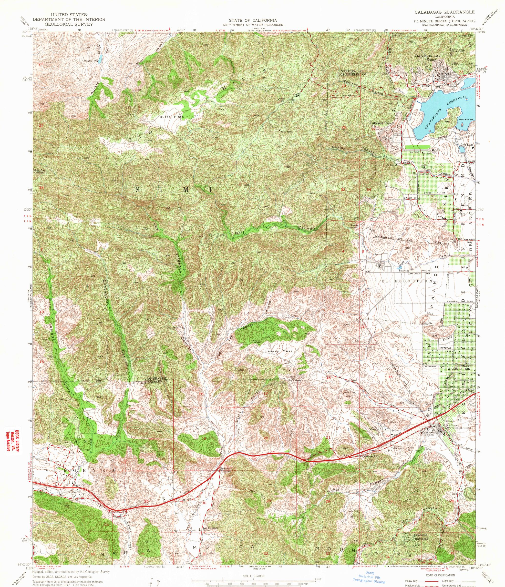
Polyconic projection. 1927 North American datum 10,000-foot grid based on California coordinate system, zones 5 and 7 Dashed land lines indicate approximate locations Dotted land lines were established by private survey 1000-meter Universal Transverse Mercator grid ticks, zone 11, shown in blue UTM GRID AND 1952 MAGNETIC NORTH DECLINATION AT CENTER OF SHEET
